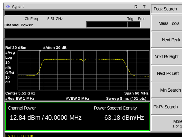
Plot 71. RF Output Power, 802.11n 40 MHz, Channel 100, MIMO
