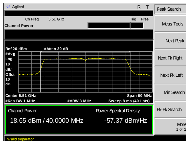
Plot 91. RF Output Power, 802.11ac 40 MHz, Channel 100, SISO
