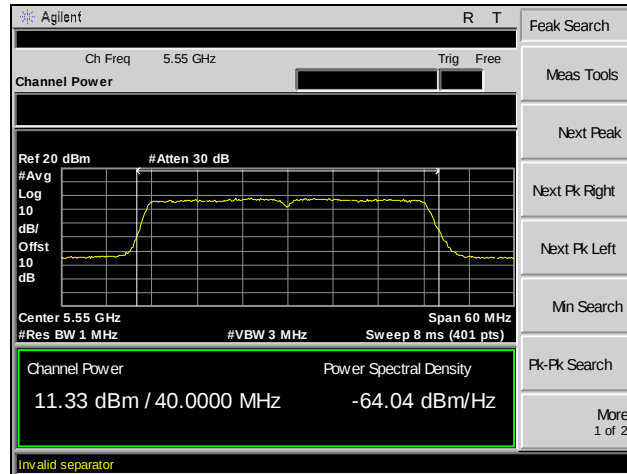
Plot 72. RF Output Power, 802.11n 40 MHz, Channel 108, MIMO
