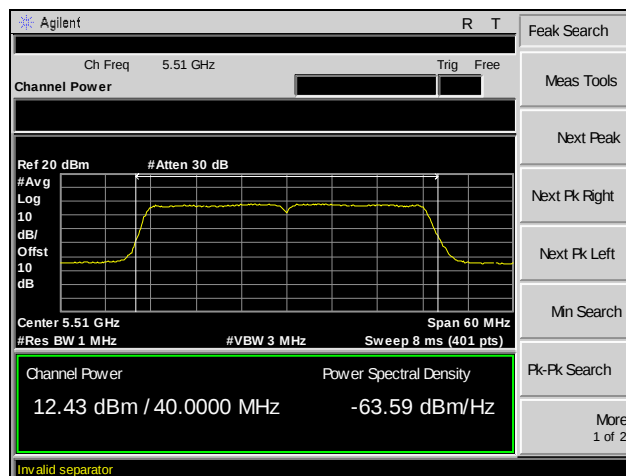
Plot 54. RF Output Power, 802.11ac 40 MHz, Channel 100, MIMO
