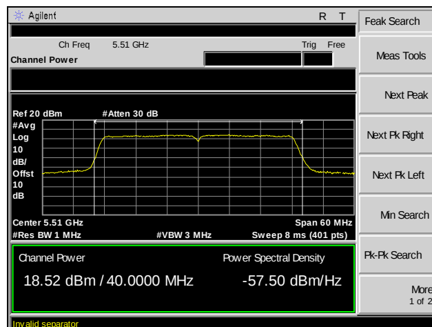
Plot 108. RF Output Power, 802.11n 40 MHz, Channel 100, SISO
