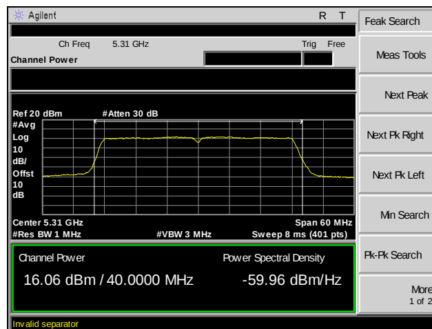
Plot 107. RF Output Power, 802.11n 40 MHz, Channel 60, SISO
