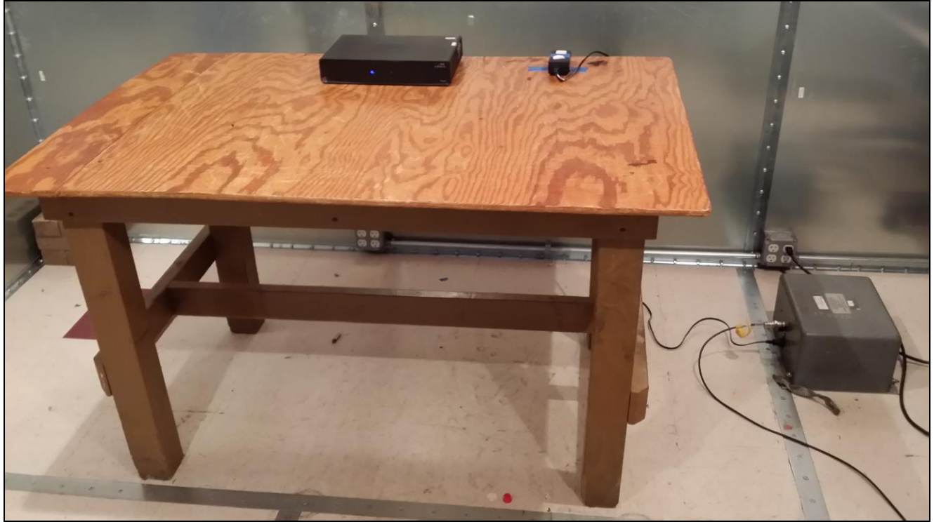
Photograph 2. Conducted Emissions, Test Setup
