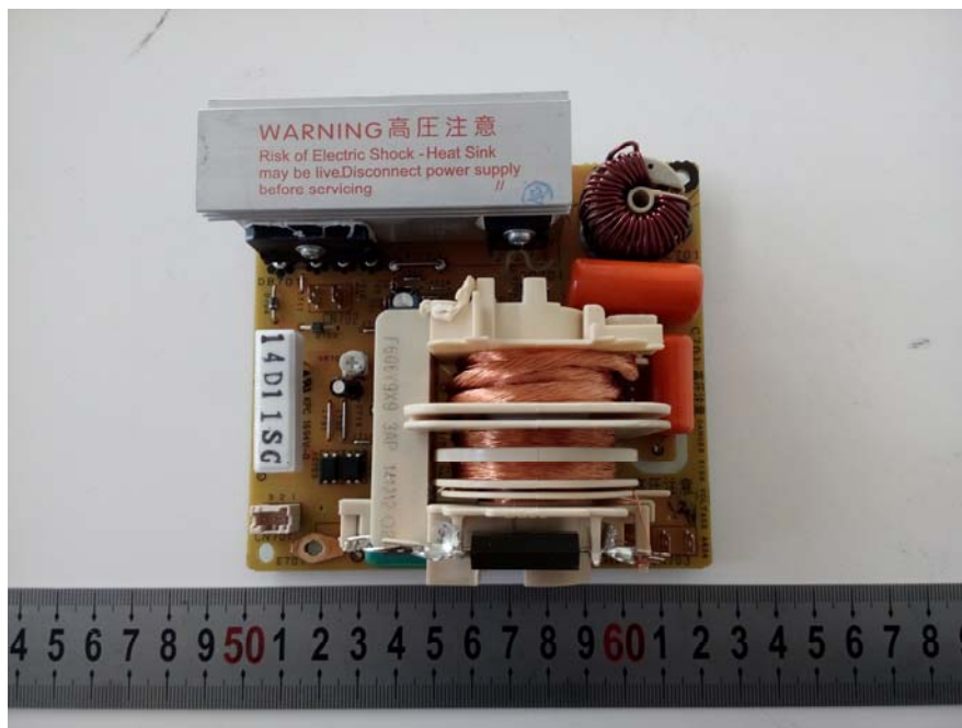
EUT - Transformer Top View
