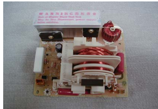
Exhibit 2-J View of Inverter Circuitry
