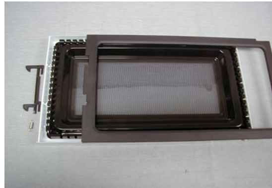
Exhibit 2-L View of Door Choke Construction
