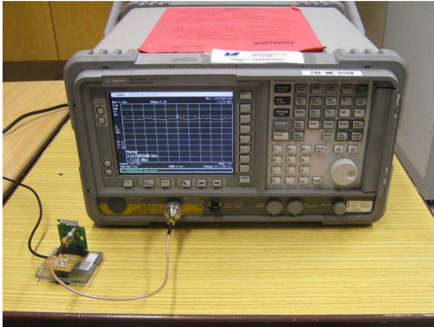
Peak Power Spectral Density Test Setup
