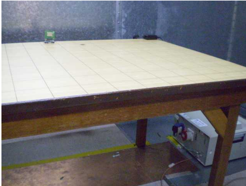
Conducted Emissions Test Setup (Front View)
