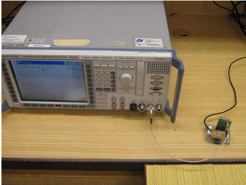
Maximum Peak Power Test Setup
