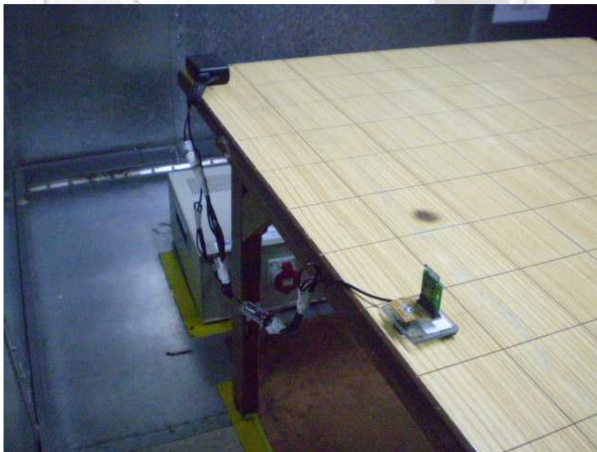
Conducted Emissions Test Setup (Rear View)
