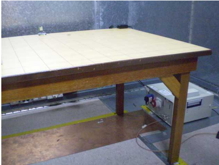
Conducted Emissions Test Setup (Front View)
