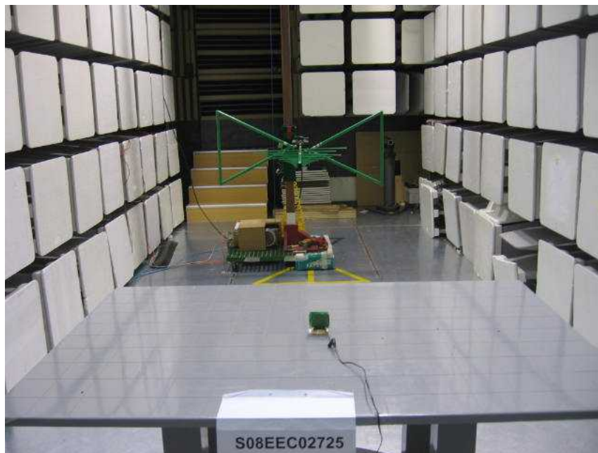
Radiated Emissions Test Setup (Rear View)
