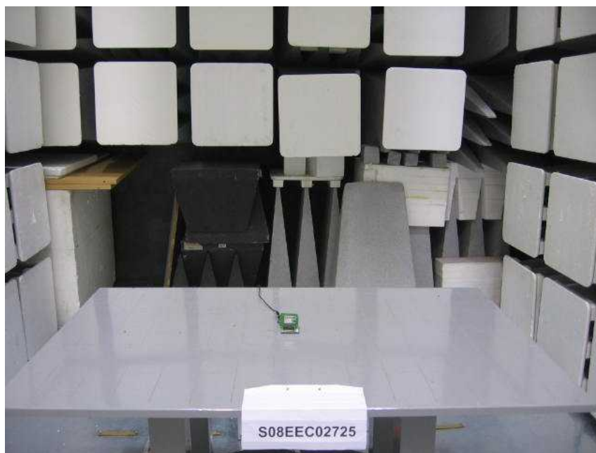
Radiated Emissions Test Setup (Front View)
