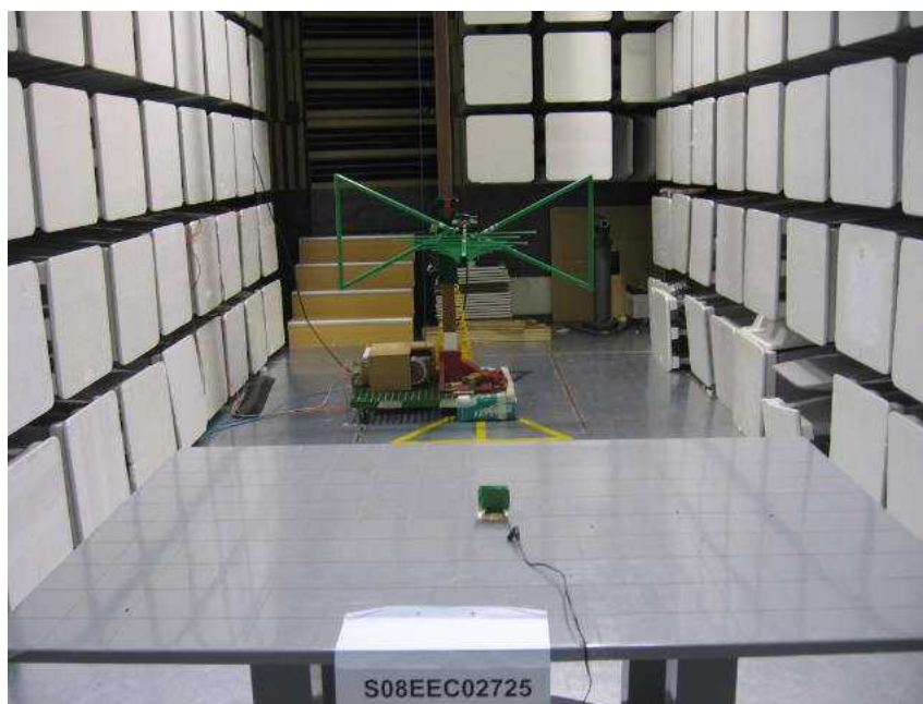
Radiated Emissions Test Setup (Rear View)
