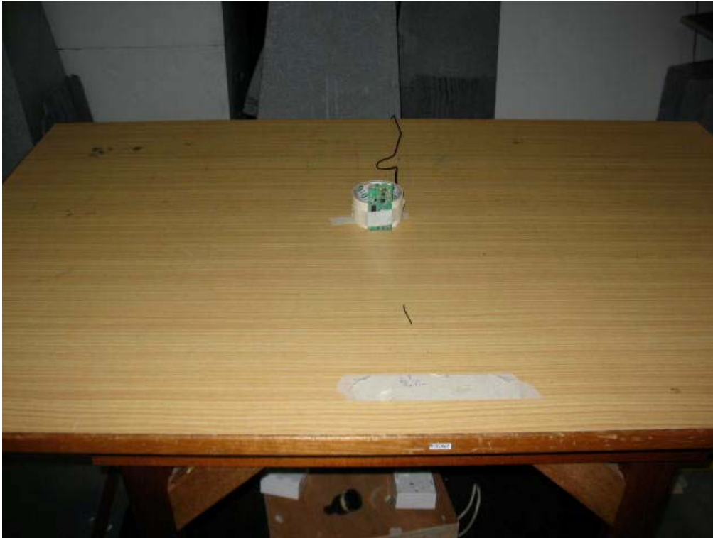
Radiated Emissions Test Setup (Front View)
