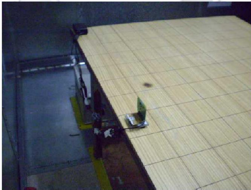
Conducted Emissions Test Setup (Rear View)
