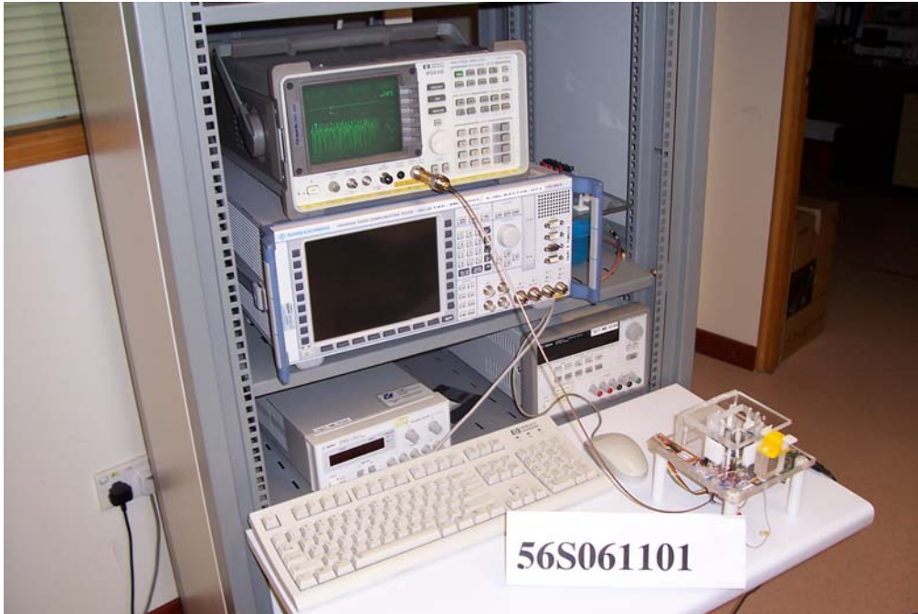
RF Conducted Spurious Emissions Test Setup
