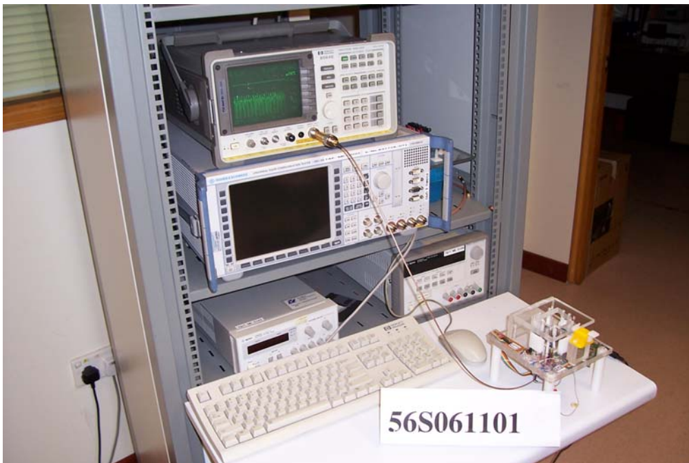
Peak Power Spectral Density Test Setup
