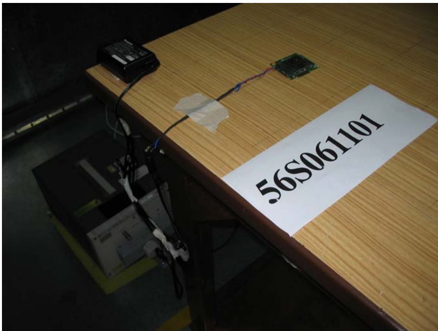
Conducted Emissions Test Setup ( Rear View )
