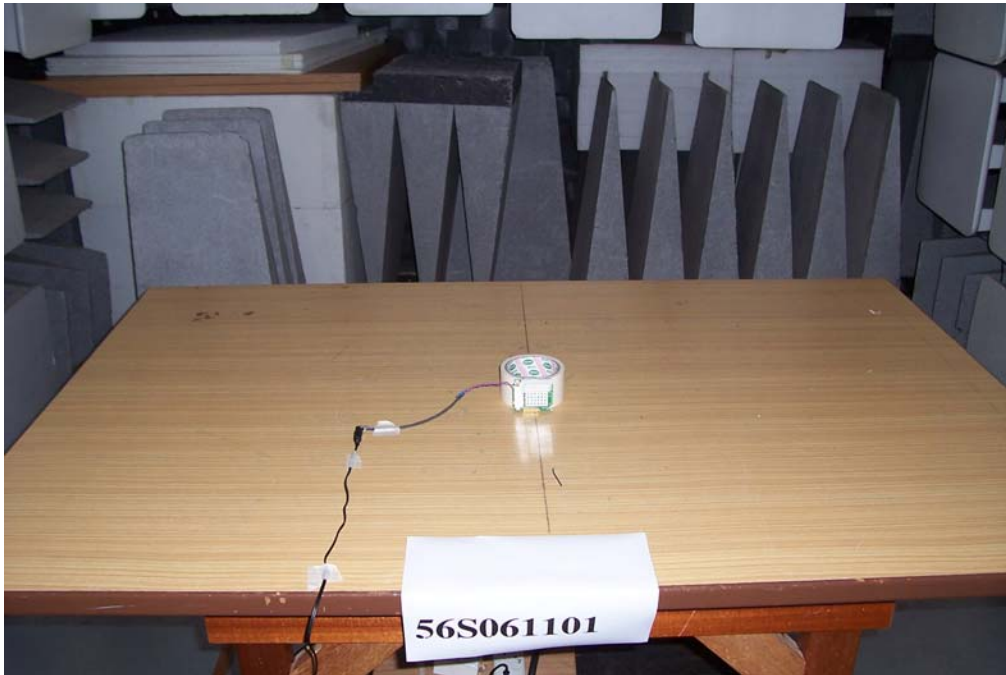
Radiated Emissions Test Setup ( Front View )
