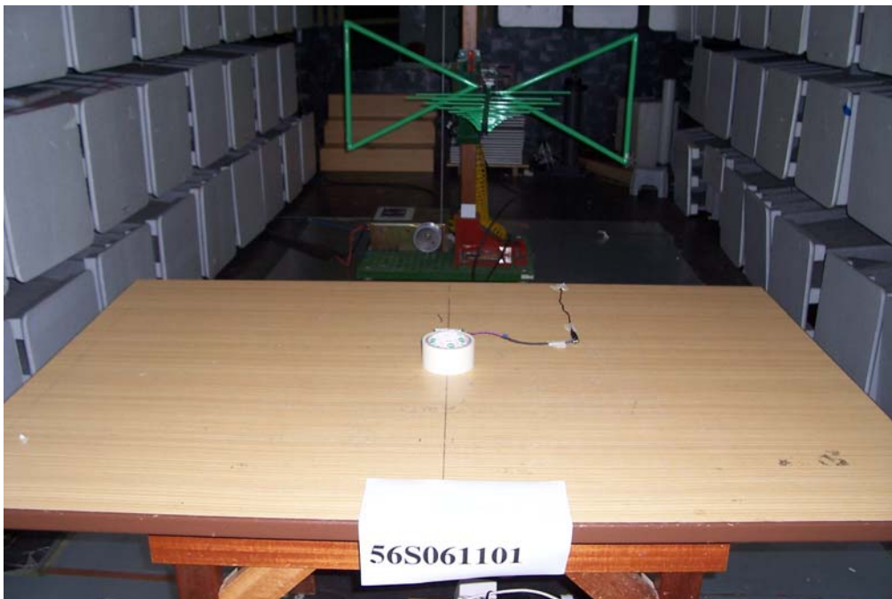
Radiated Emissions Test Setup ( Rear View )
