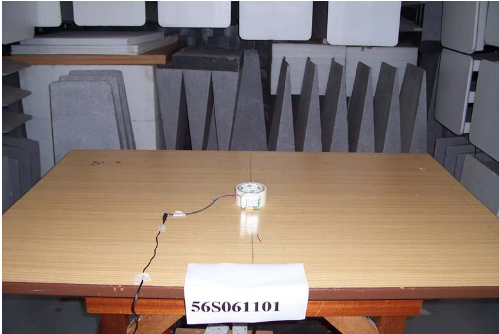
Band Edge Compliance ( Radiated ) Test Setup
