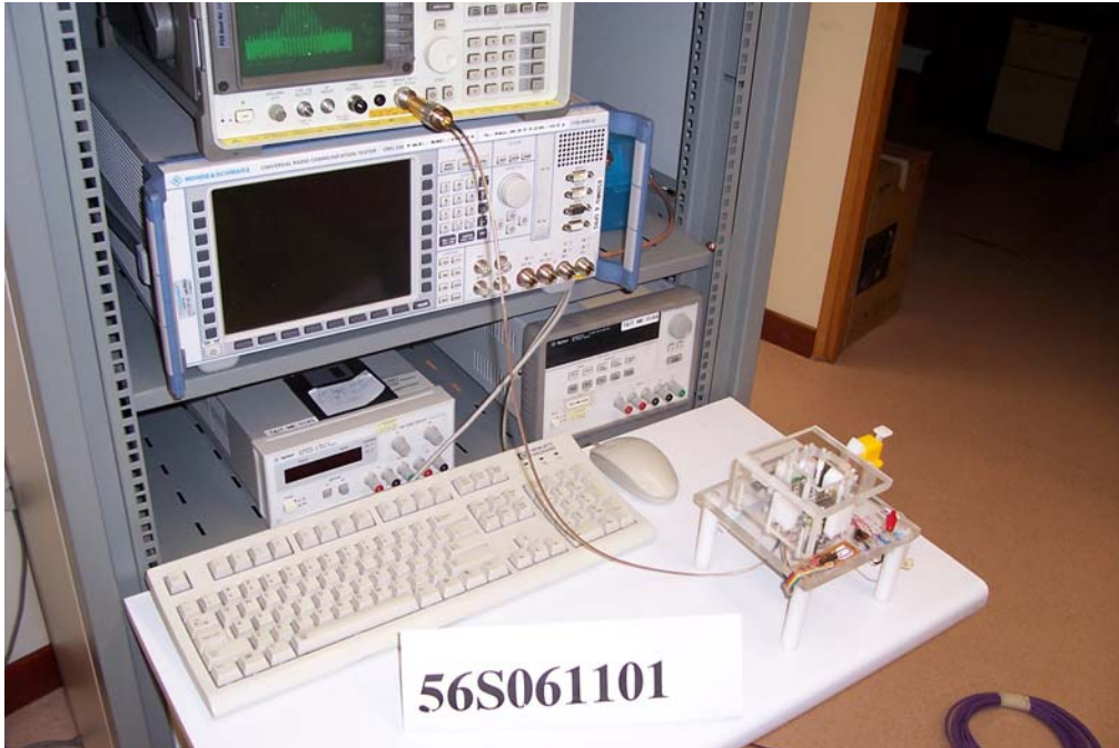
Spectrum Bandwidth ( 6 dB Bandwidth Measurement ) Test Setup
