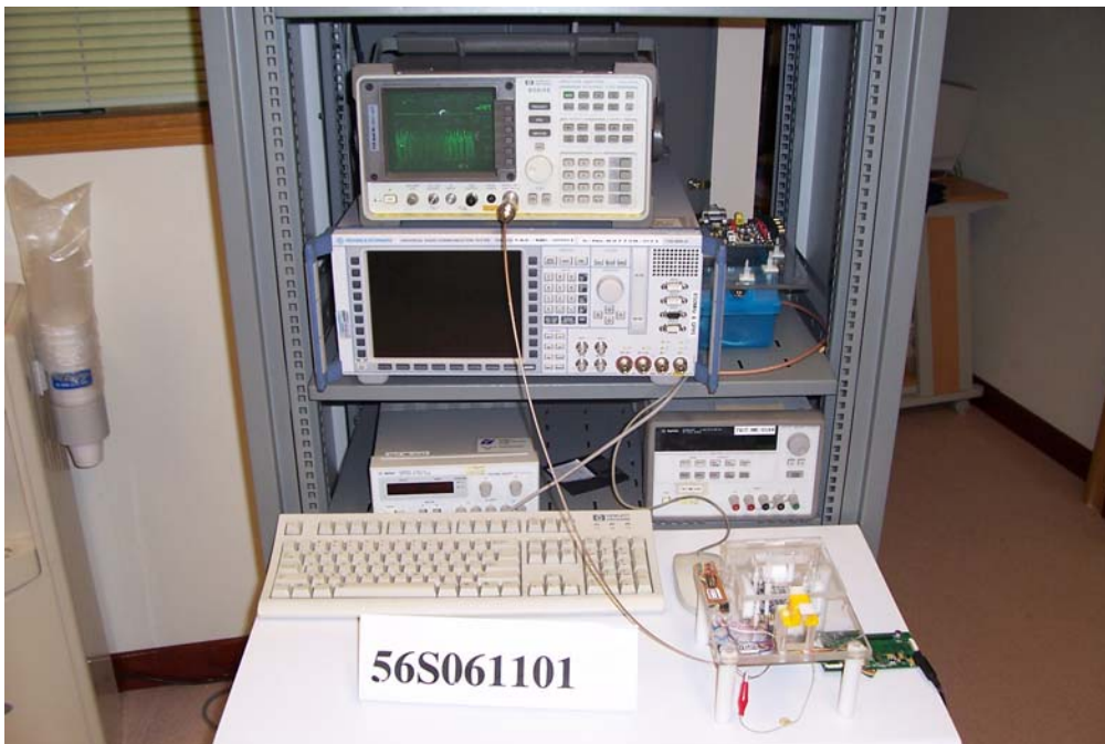
Band Edge Compliance ( Conduced ) Test Setup
