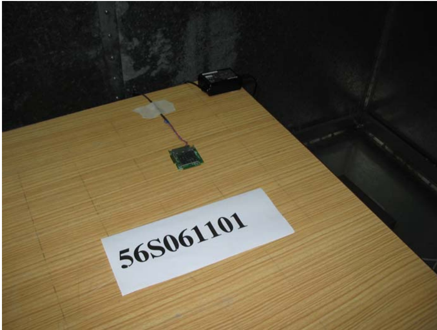
Conducted Emissions Test Setup ( Front View )
