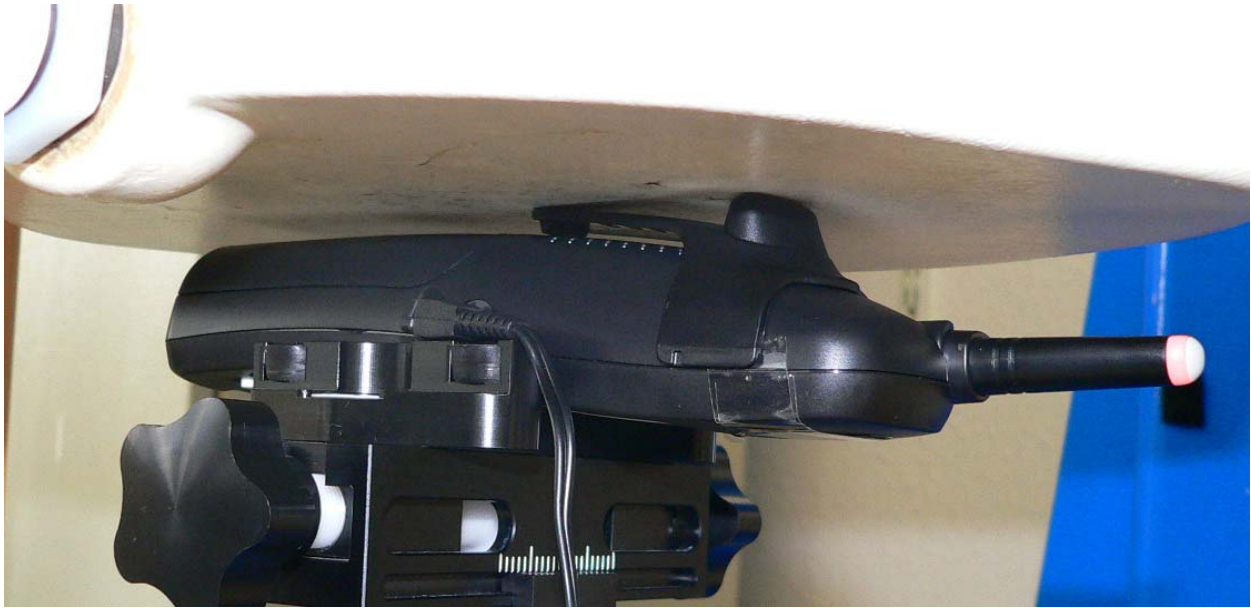
Fig. 23: Body worn, antenna 1 or antenna 2 configuration, with headset, antenna towards the phantom.
