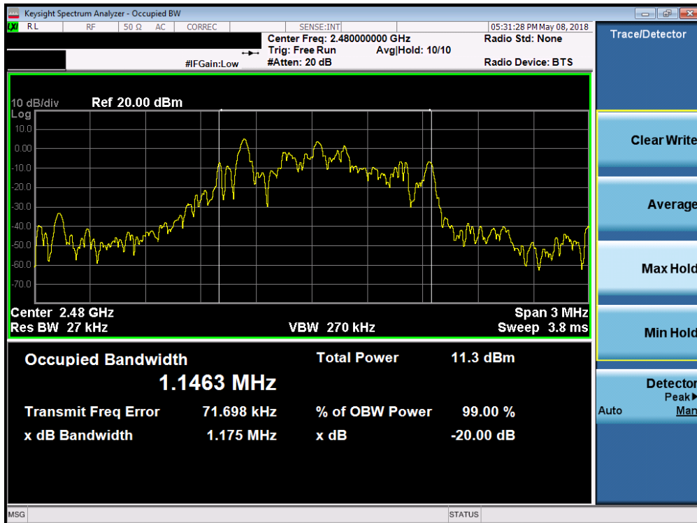
Plot 7-9. 20dB Bandwidth Plot (Bluetooth, 3Mbps – Ch. 78)
