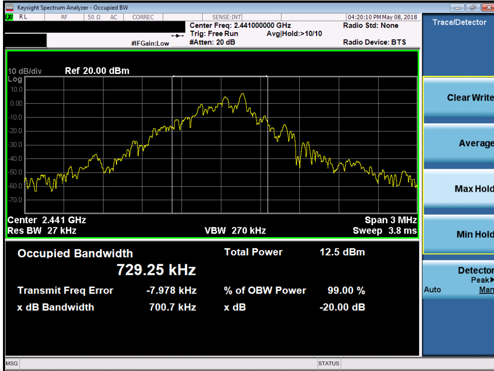
Plot 7-2. 20dB Bandwidth Plot (Bluetooth, 1Mbps – Ch. 39)
