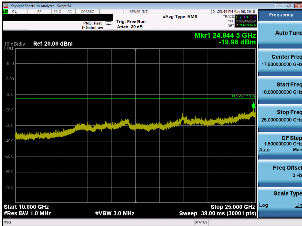
Plot 7-39. Conducted Spurious Plot (Bluetooth, 1Mbps – Ch. 39)
