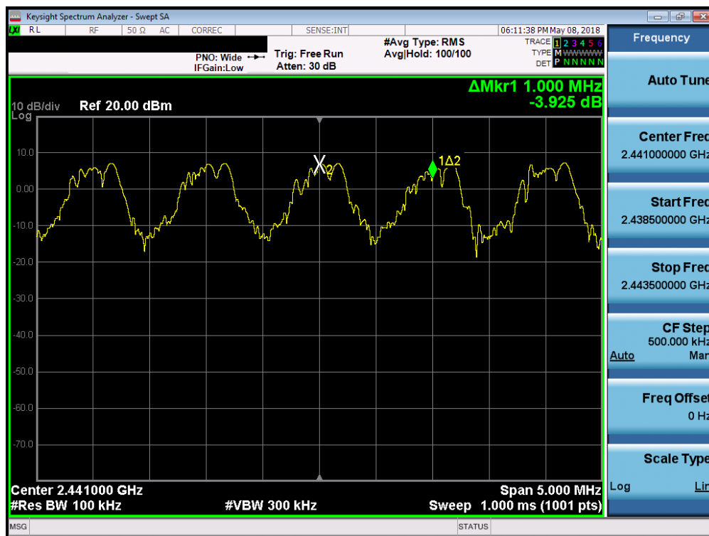
Plot 7-32. Channel Spacing Plot (Bluetooth)
