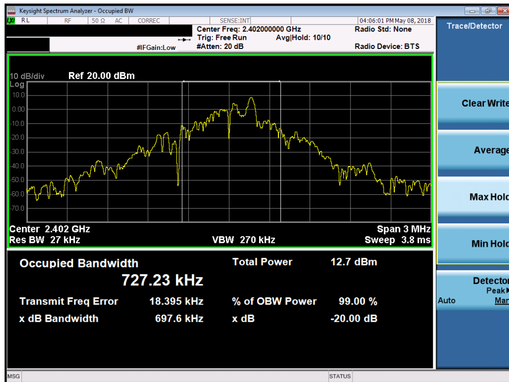
Plot 7-1. 20dB Bandwidth Plot (Bluetooth, 1Mbps – Ch. 0)
