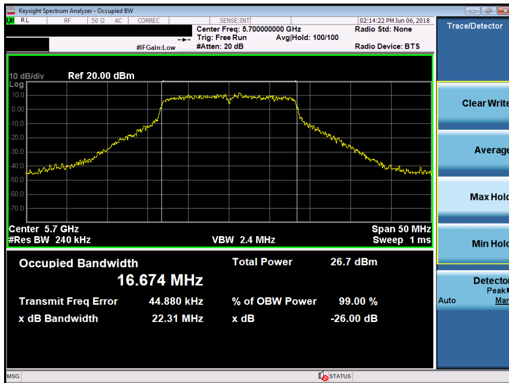
Plot 7-21. 26dB Bandwidth Plot (802.11a (UNII Band 2C) – Ch. 140)
