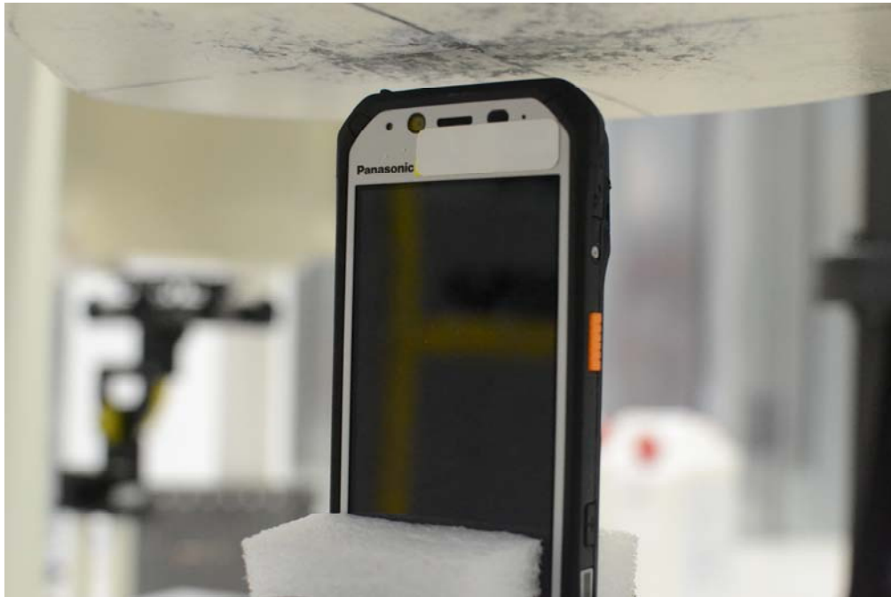
SAR Test Setup Photo 20 – Top Edge at 1.0 cm with Standard Battery
