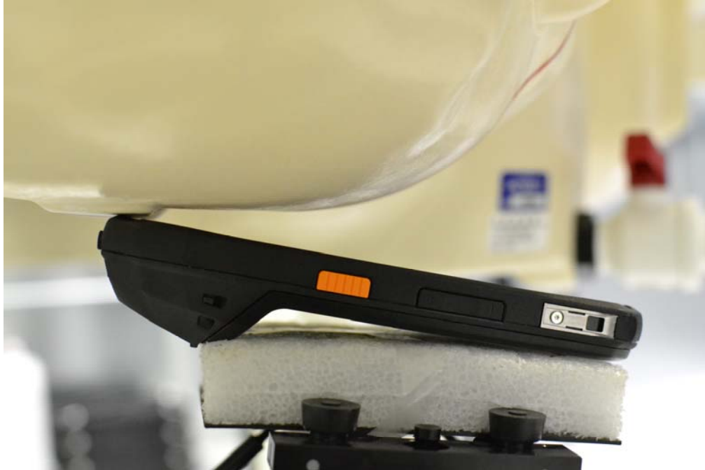
SAR Test Setup Photo 3 – Right Tilt with Standard Battery
