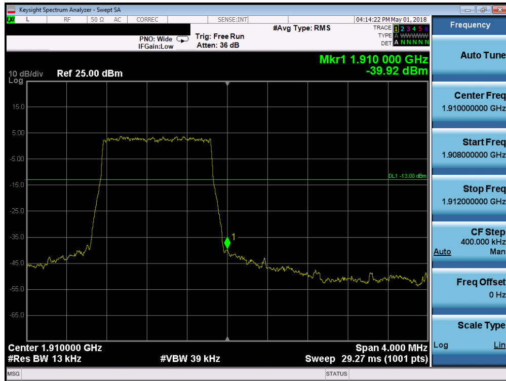
Plot 7-152. Upper Band Edge Plot (Band 2 - 1.4MHz QPSK - Full RB Configuration)
