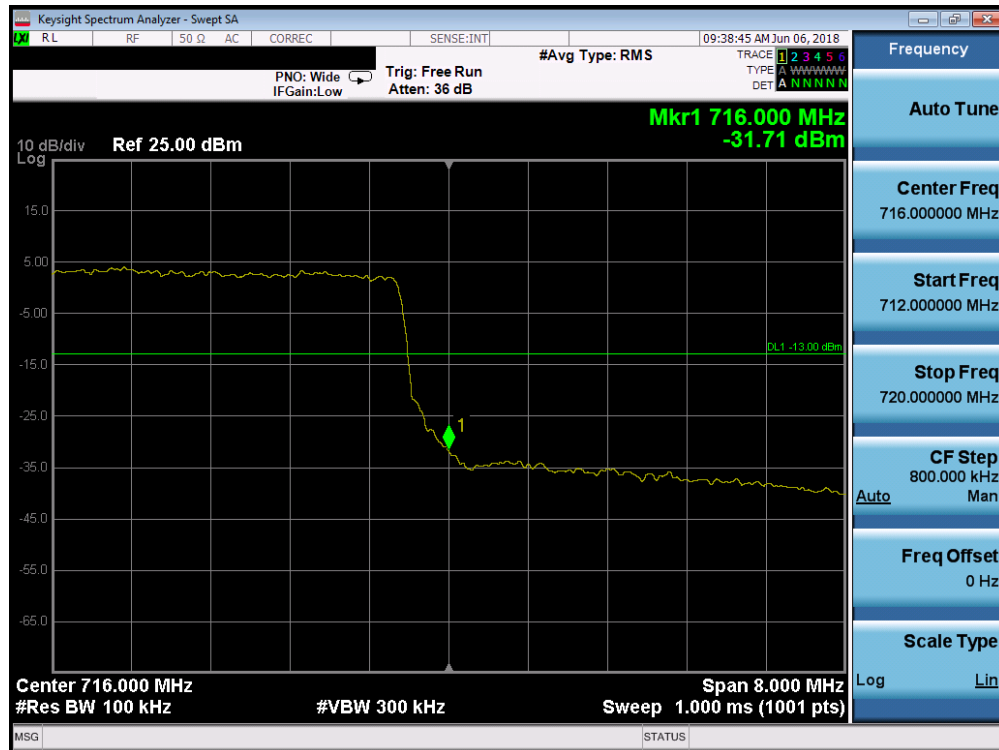
Plot 7-97. Upper Band Edge Plot (Band 12 - 10.0MHz QPSK - Full RB Configuration)
