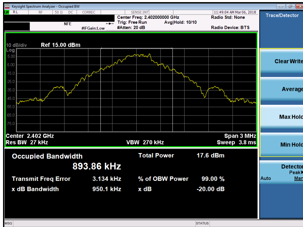
Plot 7-1. 20dB Bandwidth Plot (Bluetooth, 1Mbps – Ch. 0)
