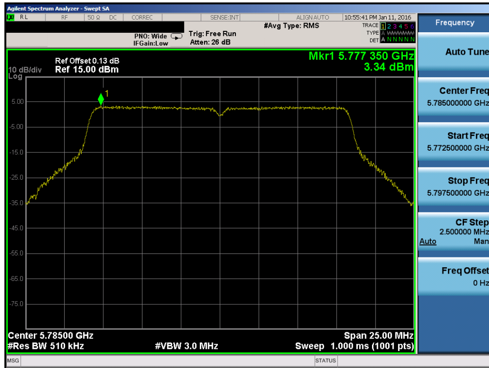
Plot 7-67. Power Spectral Density Plot (802.11a (UNII Band 3) – Ch. 157)
