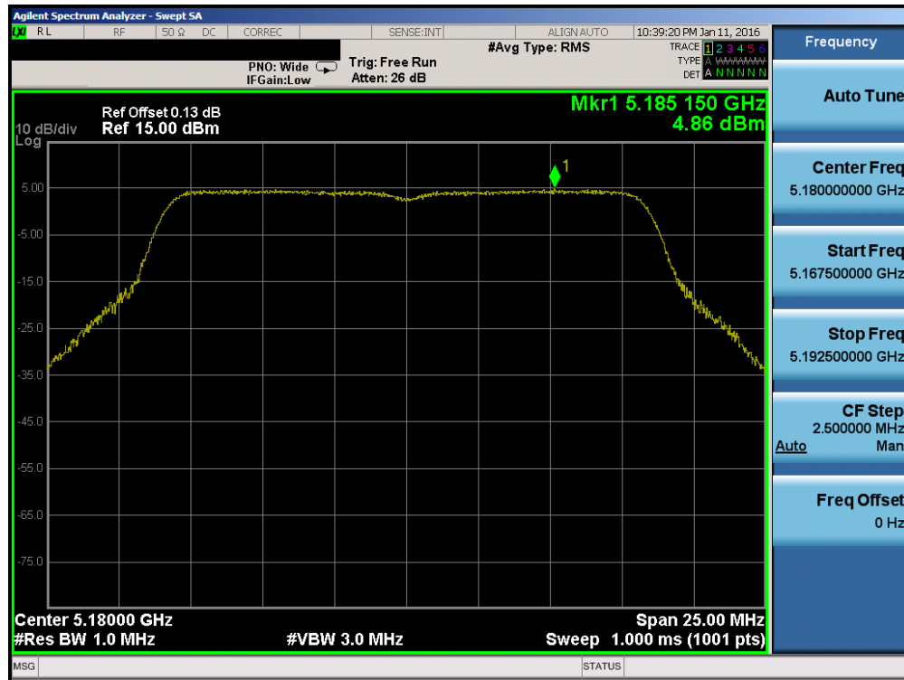
Plot 7-38. Power Spectral Density Plot (802.11a (UNII Band 1) – Ch. 36)
