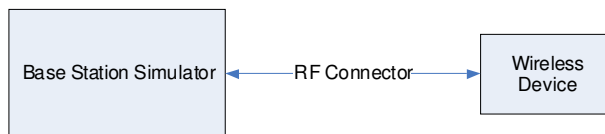
Figure 9-1 Power Measurement Setup
