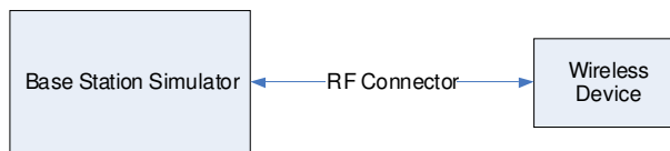
Figure 9-2 Power Measurement Setup
