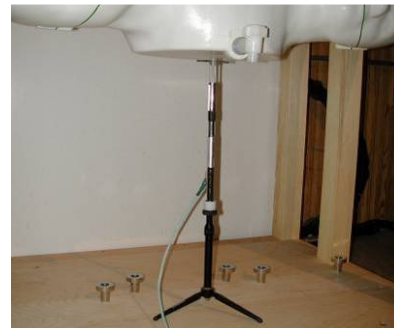
Figure 10-2 System Verification Setup Photo
