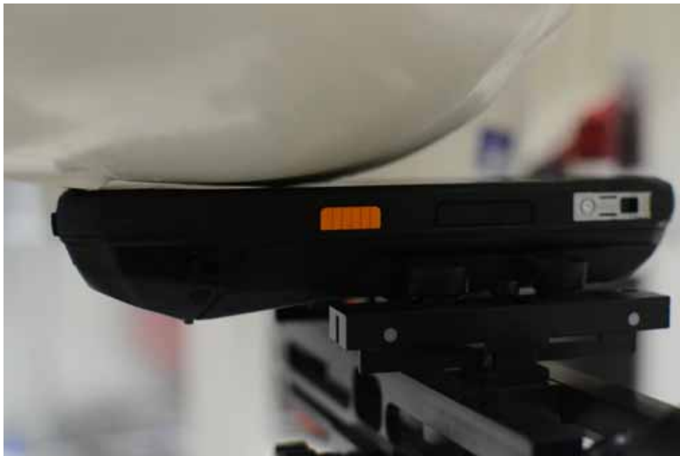
SAR Test Setup Photo 2 – Right Cheek with L-Battery
