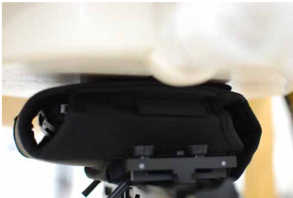
SAR Test Setup Photo 18 – Front Side at 0.0 cm with L-Battery and Body Holster Accessory
