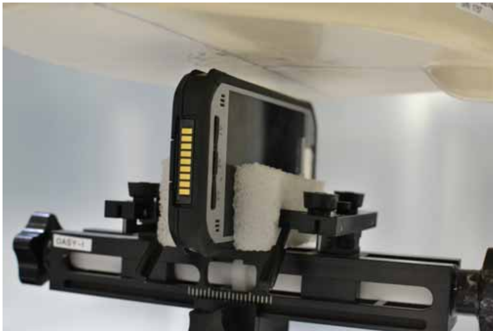
SAR Test Setup Photo 24 – Left Edge at 1.0 cm with Standard Battery
