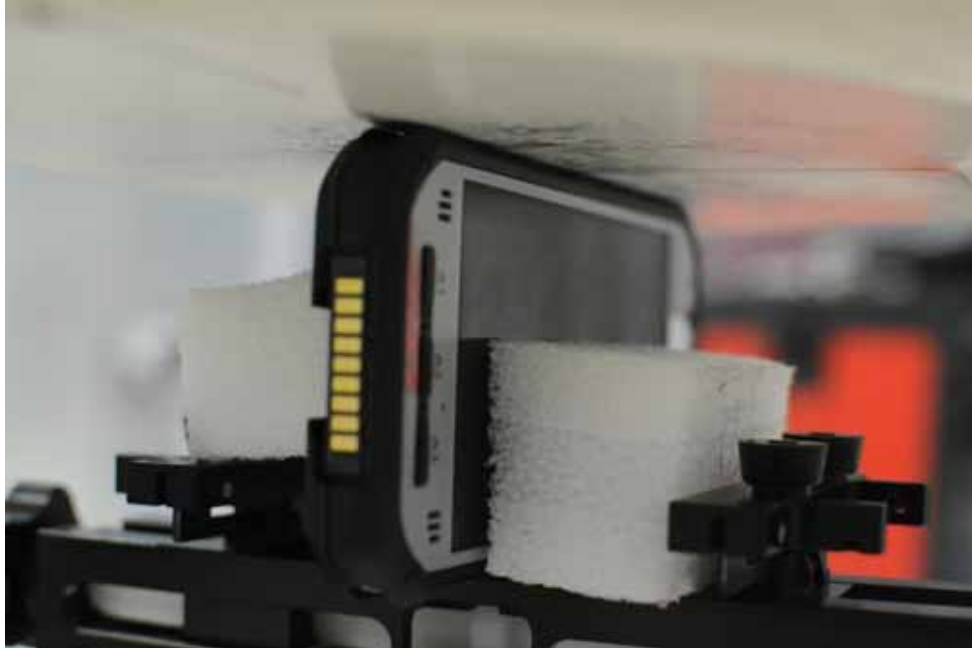
SAR Test Setup Photo 25 – Left Edge at 0.0 cm with Standard Battery
