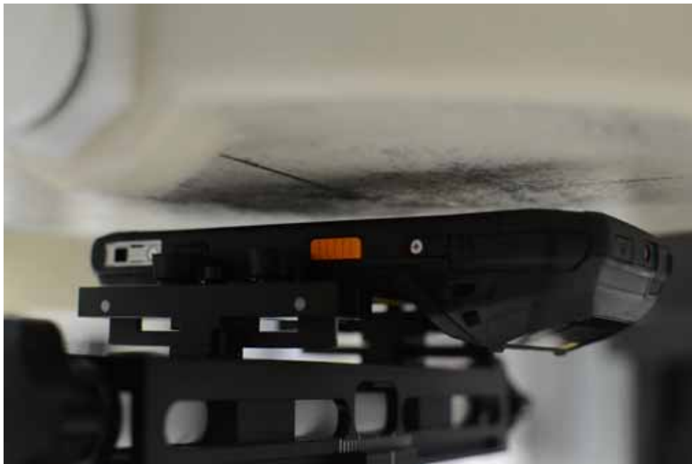
SAR Test Setup Photo 14 – Front Side at 1.0 cm with Standard Battery
