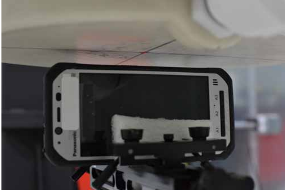
SAR Test Setup Photo 23 – Right Edge at 1.0 cm with Standard Battery
