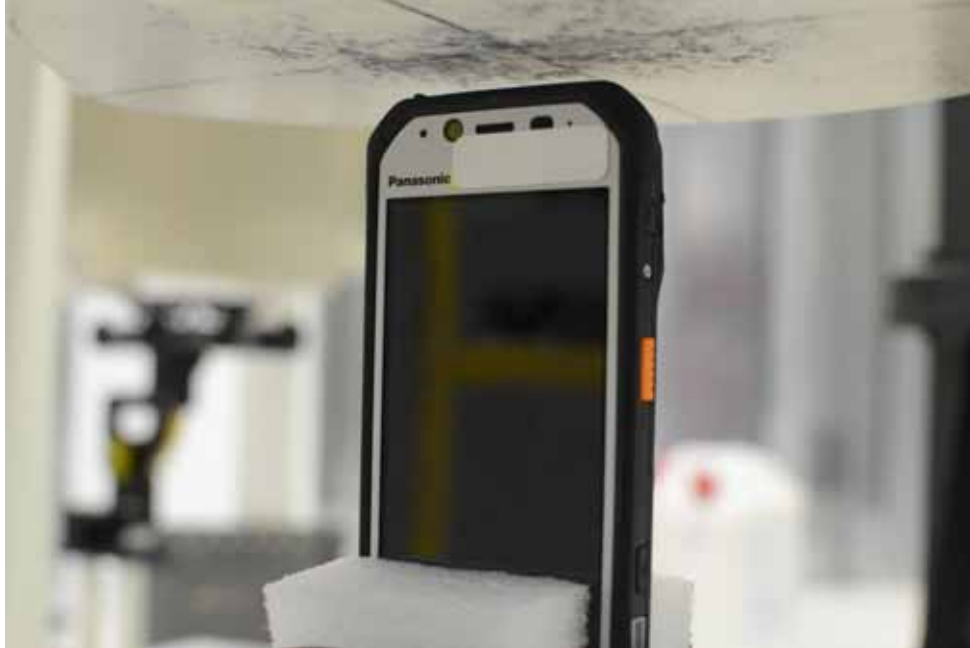
SAR Test Setup Photo 19 – Top Edge at 1.0 cm with Standard Battery
