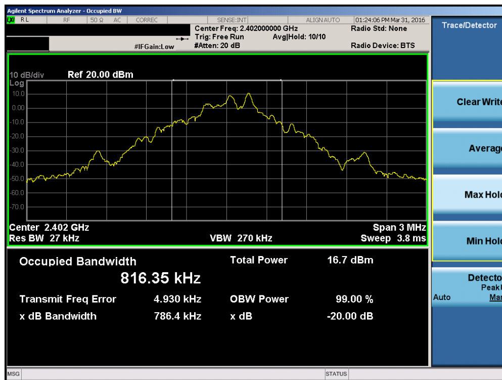
Plot 7-1. 20dB Bandwidth Plot (Bluetooth, 1Mbps – Ch. 0)
