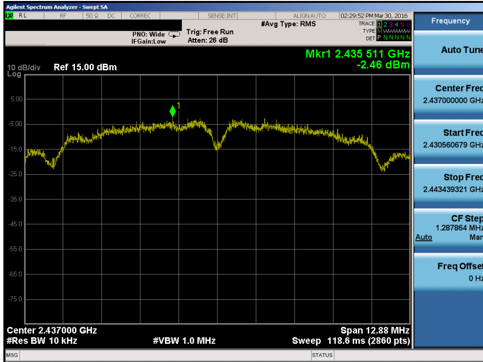
Plot 7-11. Power Spectral Density Plot (802.11b – Ch. 6)
