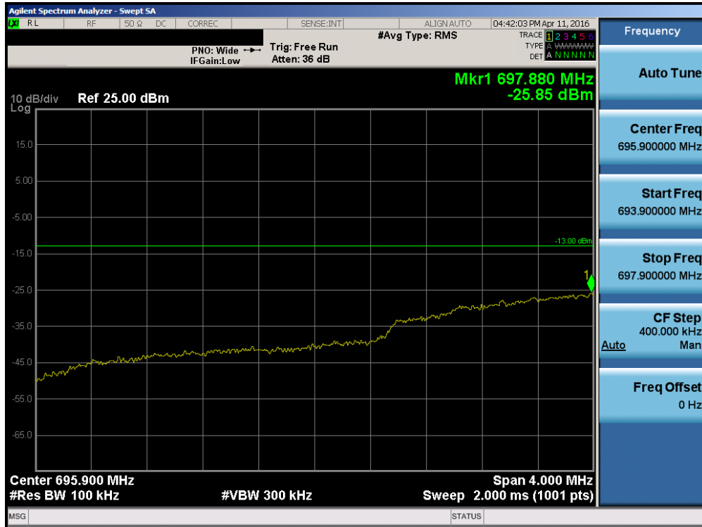
Plot 7-89. Lower Extended Band Edge Plot (Band 12 – 3.0MHz QPSK – RB Size 15)
