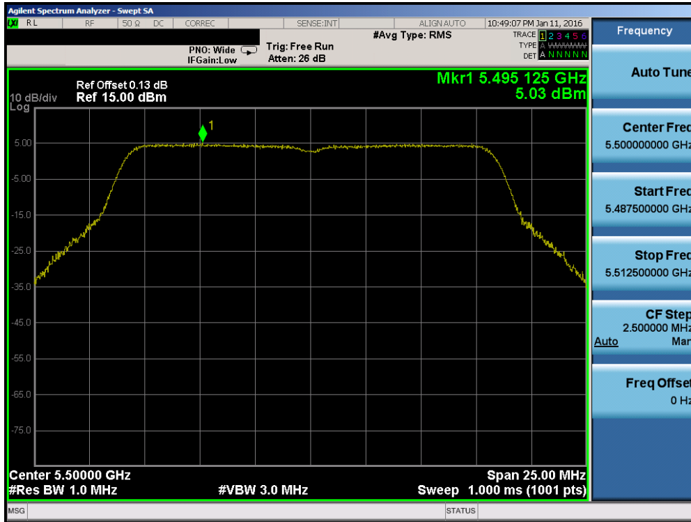
Plot 7-57. Power Spectral Density Plot (802.11a (UNII Band 2C) – Ch. 100)
