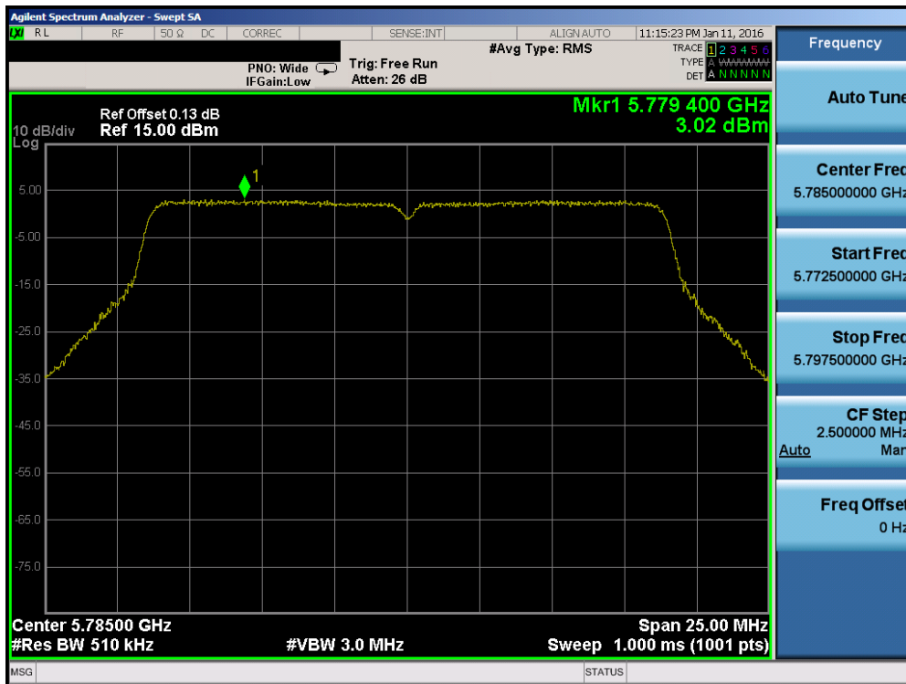
Plot 7-72. Power Spectral Density Plot (20MHz BW 802.11n (UNII Band 3) – Ch. 157)
