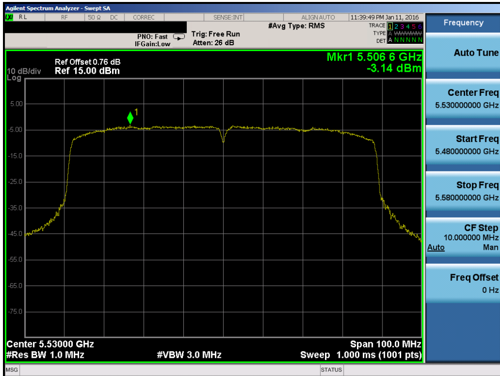
Plot 7-66. Power Spectral Density Plot (80MHz BW 802.11ac (UNII Band 2C) – Ch. 106)
