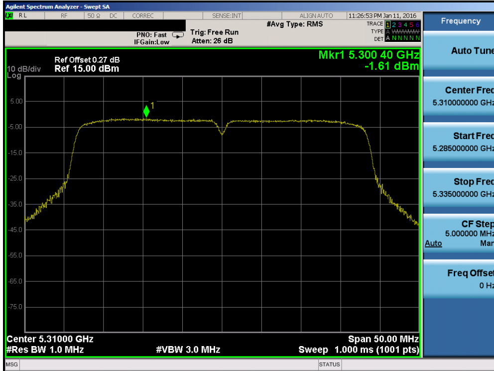
Plot 7-55. Power Spectral Density Plot (40MHz BW 802.11n (UNII Band 2A) – Ch. 62)
