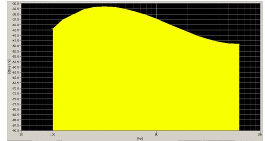
Figure 5-4 Spectral Characteristic of full P.50
