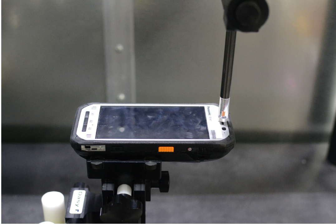
Figure 14-3 Test Setup for Wireless Device (L-Battery)
