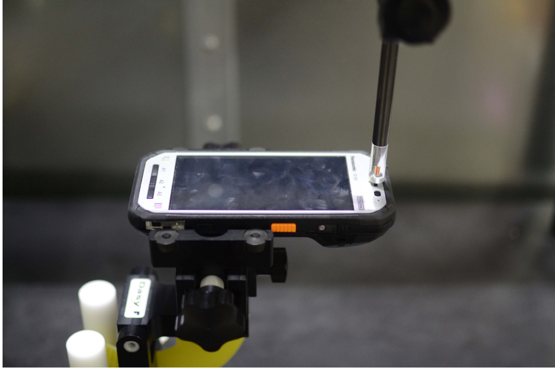
Figure 14-1 Test Setup for Wireless Device (Standard Battery)
