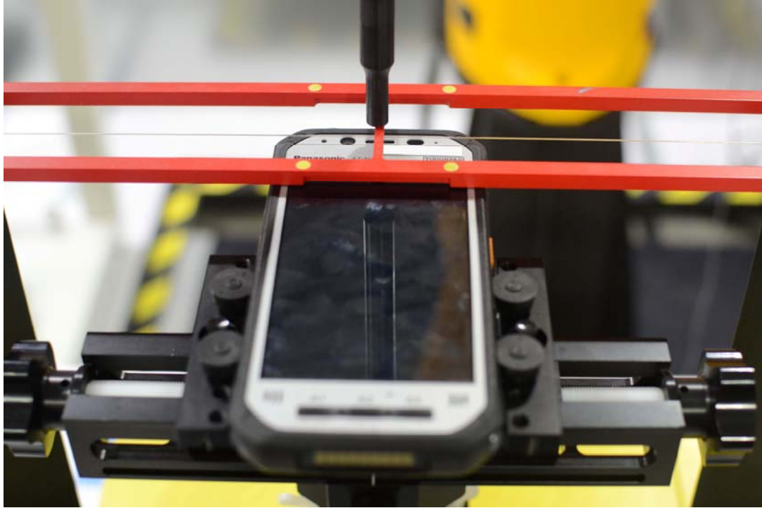
Figure 18-1 Ear Reference Point HAC Phantom Alignment (Standard Battery)
