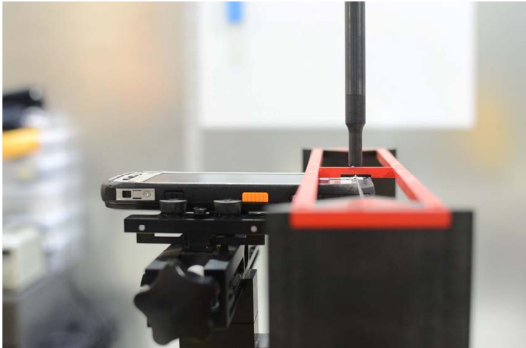
Figure 18-2 HAC Phantom Plane Alignment (Standard Battery)
