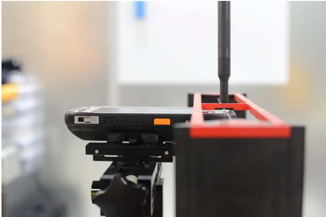
Figure 18-4 HAC Phantom Plane Alignment (L-Battery Accessory)
