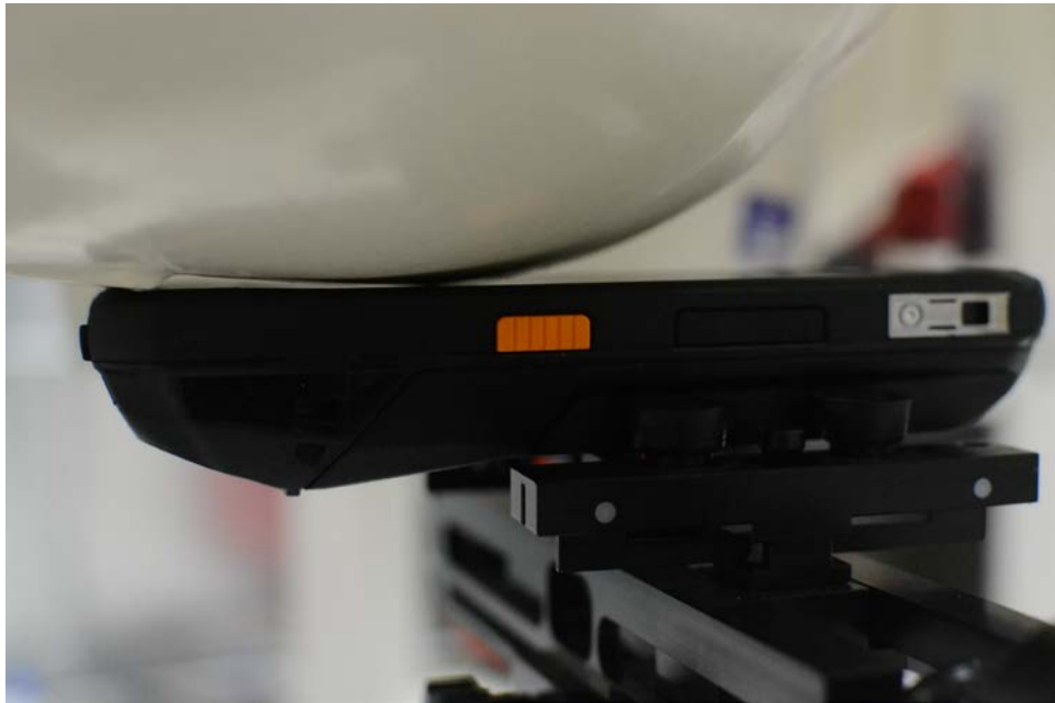
SAR Test Setup Photo 2: Right Cheek L-Battery
