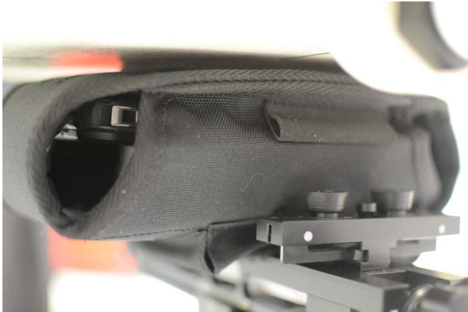
SAR Test Setup Photo 14: Front Side at 0.0 cm with Standard Battery and Body Holster Accessory
