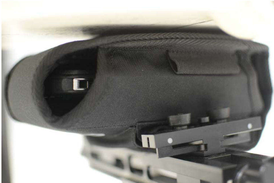
SAR Test Setup Photo 10: Back Side at 0.0 cm with Standard Battery and Body Holster Accessory
