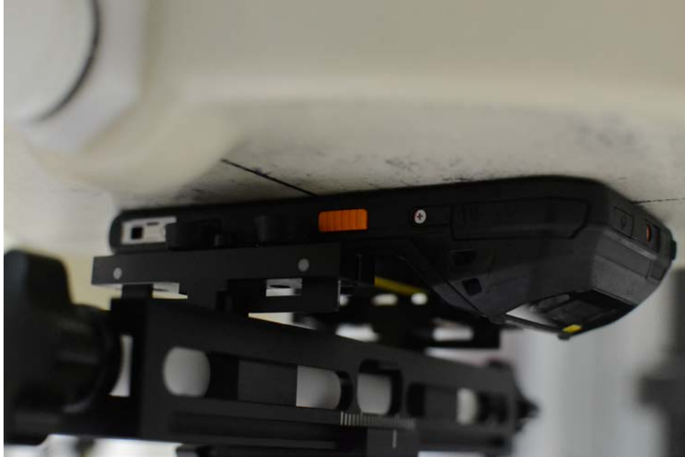
SAR Test Setup Photo 13: Front Side at 0.0 cm with Standard Battery
