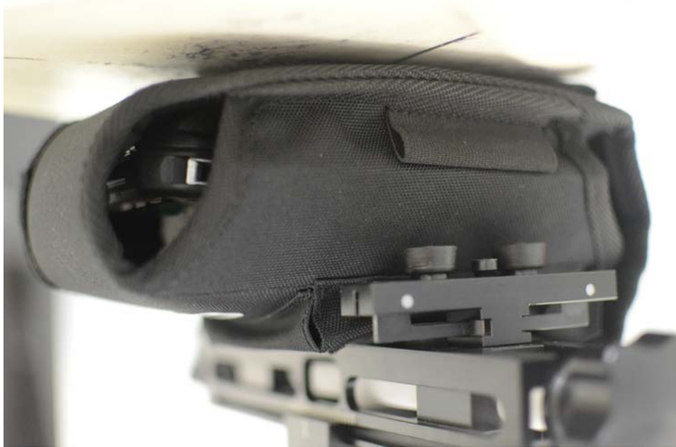
SAR Test Setup Photo 11: Back Side at 0.0 cm with L-Battery and Body Holster Accessory
