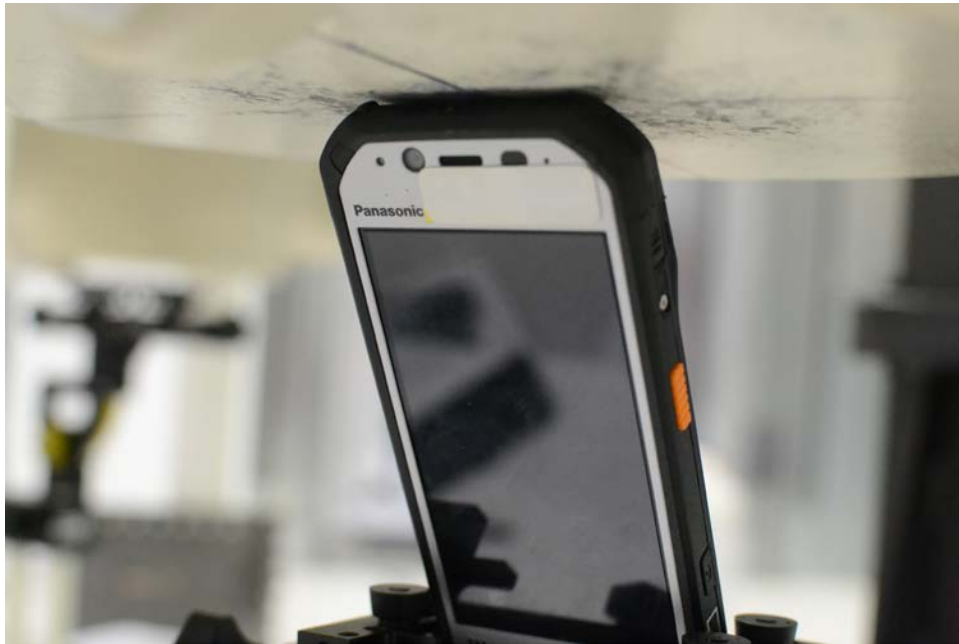
SAR Test Setup Photo 16: Top Edge (Tilt) at 0.0 cm with Standard Battery
