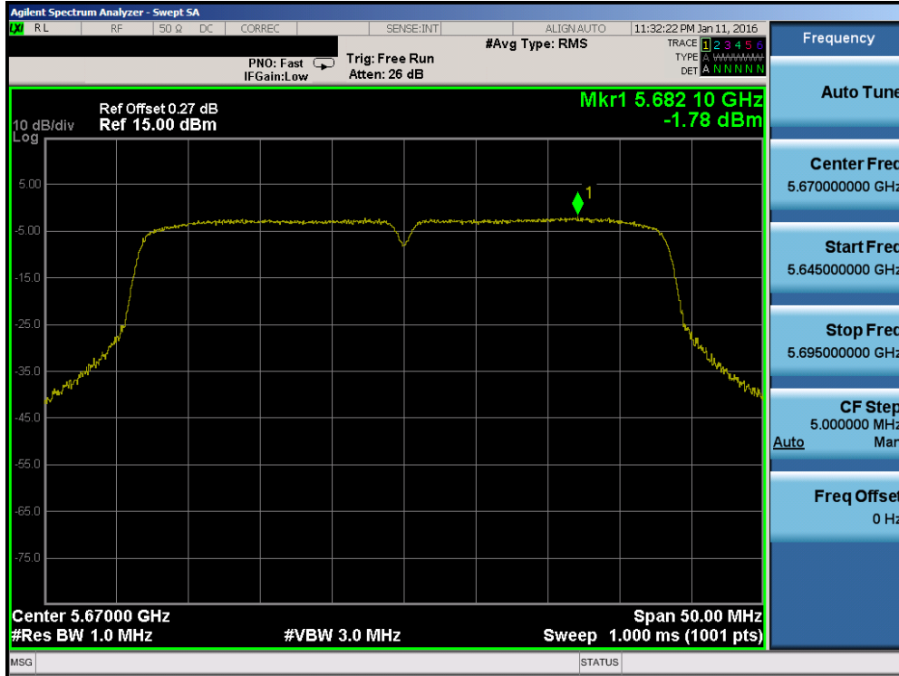
Plot 7-65. Power Spectral Density Plot (40MHz BW 802.11n (UNII Band 2C) – Ch. 134)
