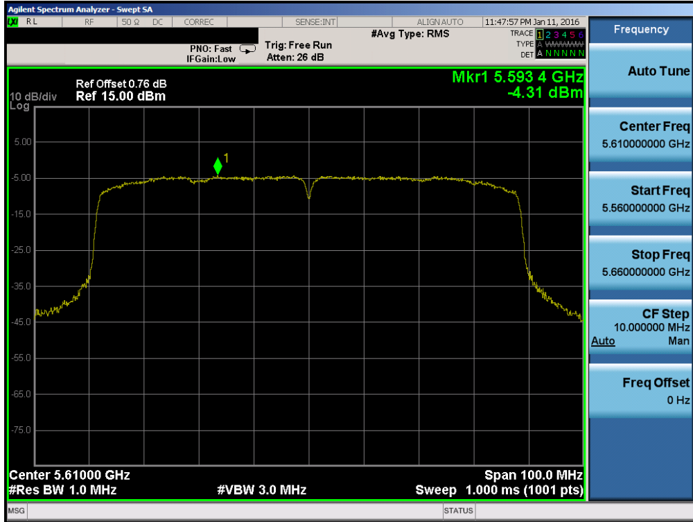
Plot 7-67. Power Spectral Density Plot (80MHz BW 802.11ac (UNII Band 2C) – Ch. 122)
