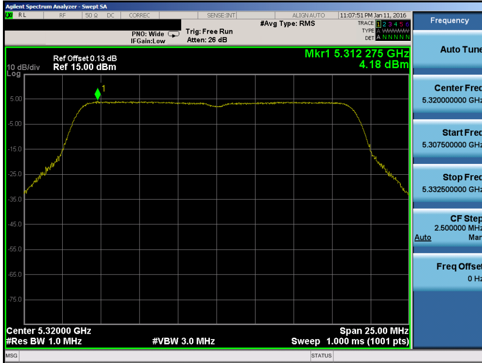
Plot 7-53. Power Spectral Density Plot (20MHz BW 802.11n (UNII Band 2A) – Ch. 64)
