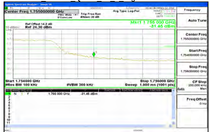
Band4 10MHz QPSK 50 0 HighCH20350-1750
