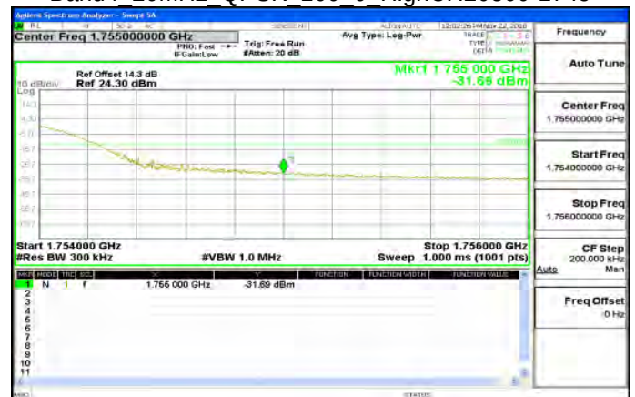
Band4 20MHz QPSK 100 0 HighCH20300-1745
