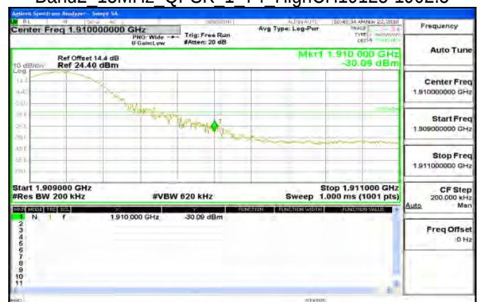
Band2 15MHz QPSK 1 74 HighCH19125-1902.5
