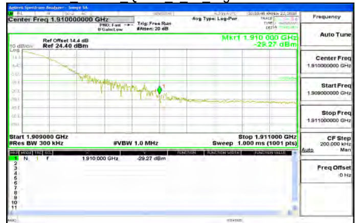
Band2 20MHz QPSK 1 99 HighCH19100-1900
