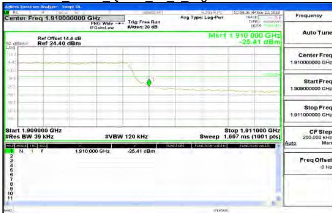
Band2 3MHz QPSK 15 0 HighCH19185-1908.5
