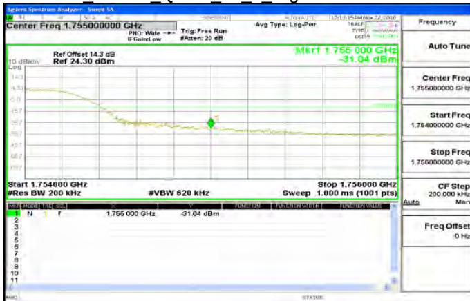
Band4 15MHz QPSK 75 0 HighCH20325-1747.5
