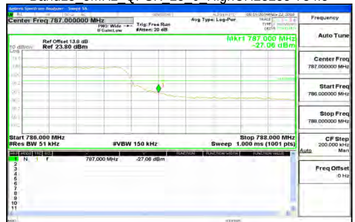
Band13 5MHz QPSK 25 0 HighCH23255-784.5
