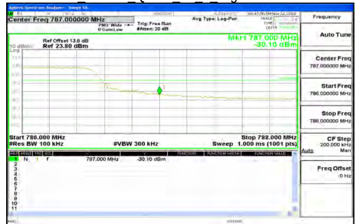
Band13 10MHz QPSK 50 0 HighCH23230-782
