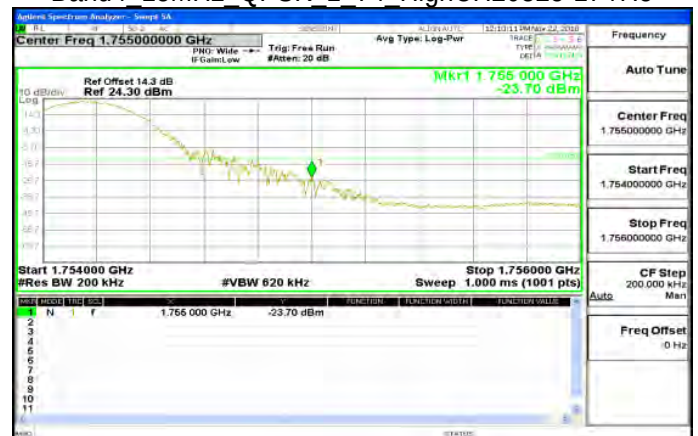
Band4 15MHz QPSK 1 74 HighCH20325-1747.5
