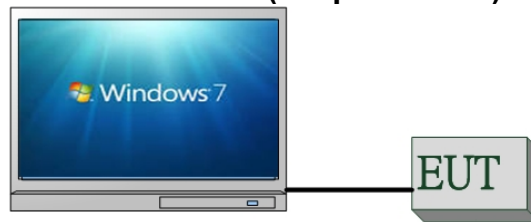
Fig.2-2 Conducted Emission (AC power line) Configuration
