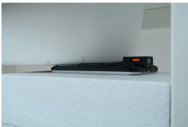
Bottom Face, Test Separation 0 mm
