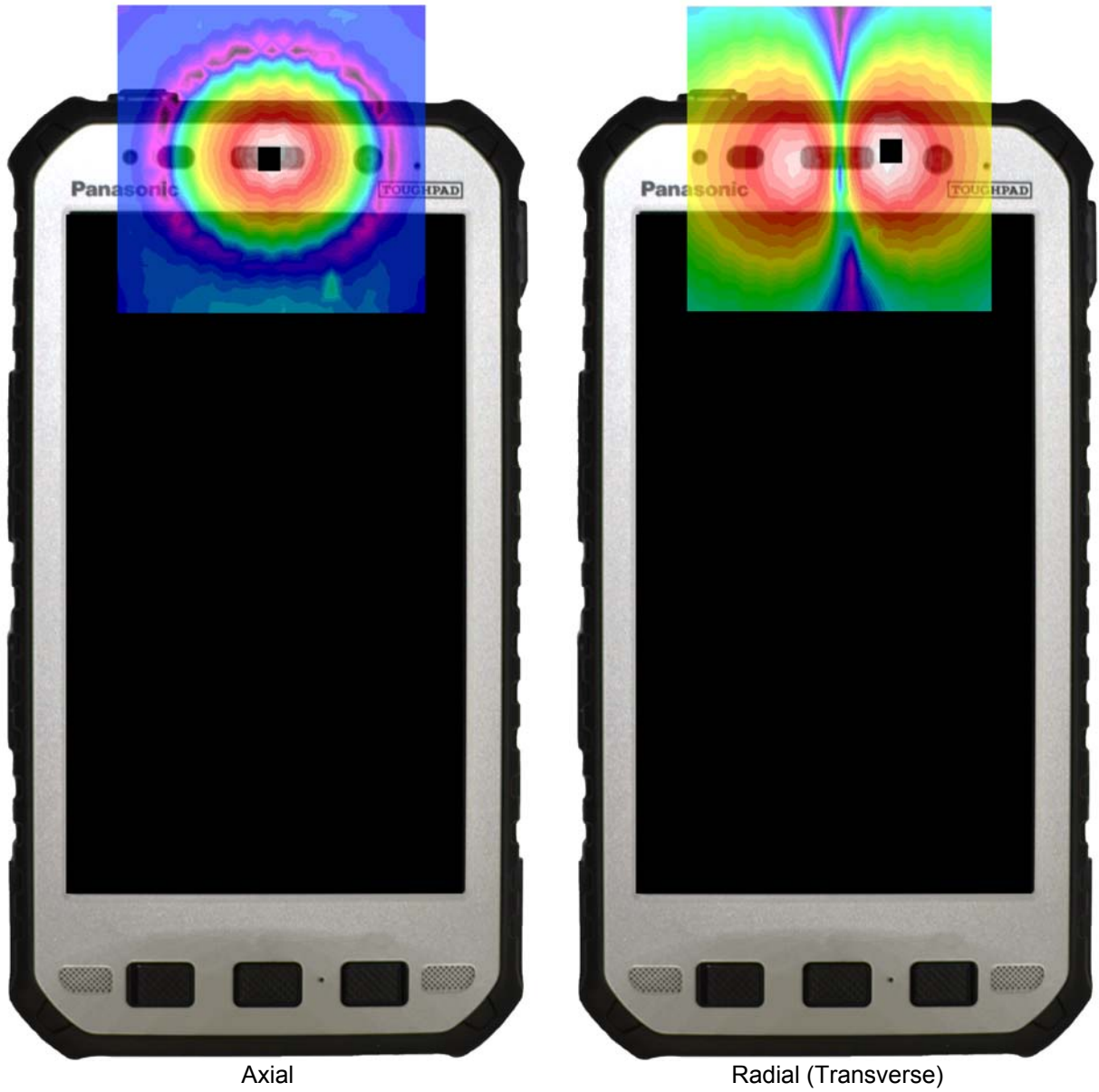
Figure 14-3 T-Coil Scan Overlay Magnetic Field Distributions
