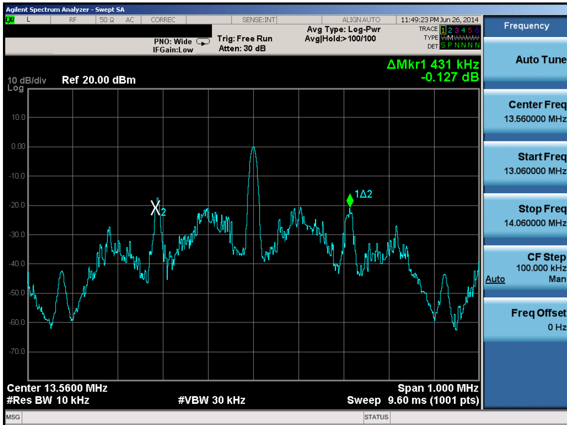
Figure 8-2. 20dB Bandwidth Plot
