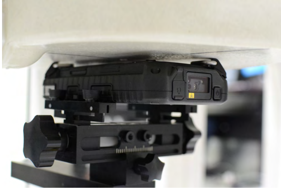
SAR Test Setup Photo 7: Back Side at 0.0 cm with Hand Strap Accessory (Top-Right)
