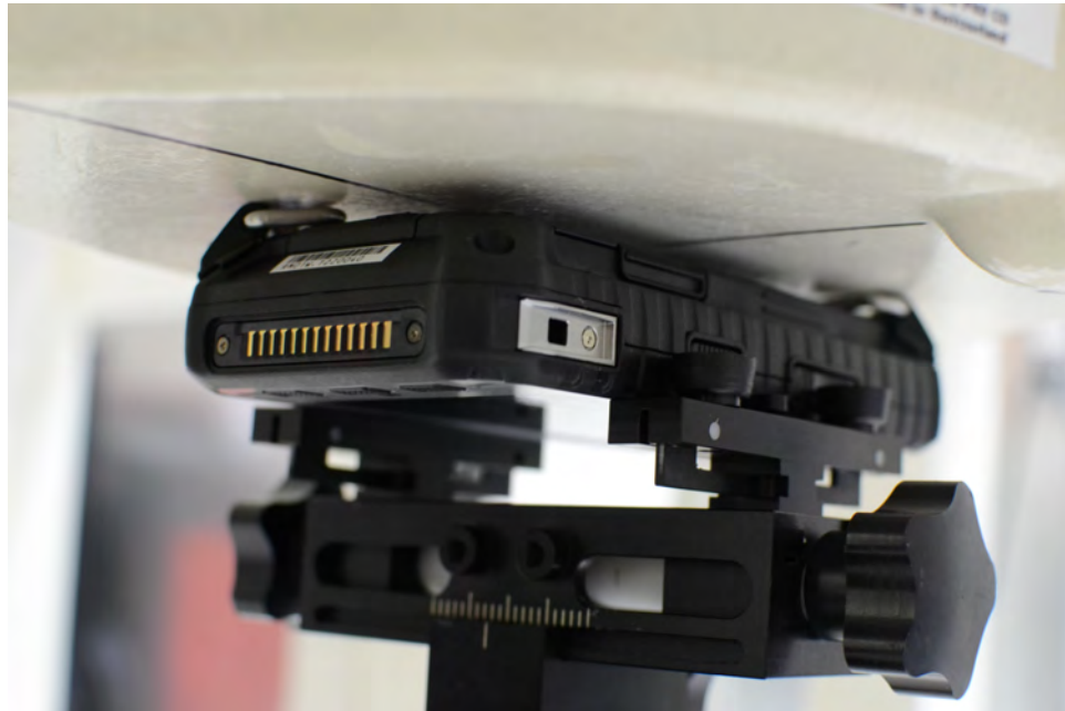
SAR Test Setup Photo 8: Back Side at 0.0 cm with Hand Strap Accessory (Top-Left)
