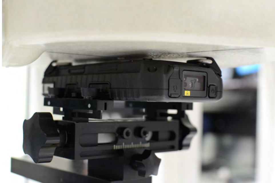
SAR Test Setup Photo 7: Back Side at 0.0 cm with Hand Strap Accessories (Top-Right)
