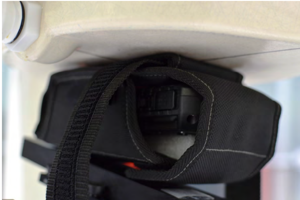
SAR Test Setup Photo 12: Front Side at 0.0 cm with Body Holster Accessory
