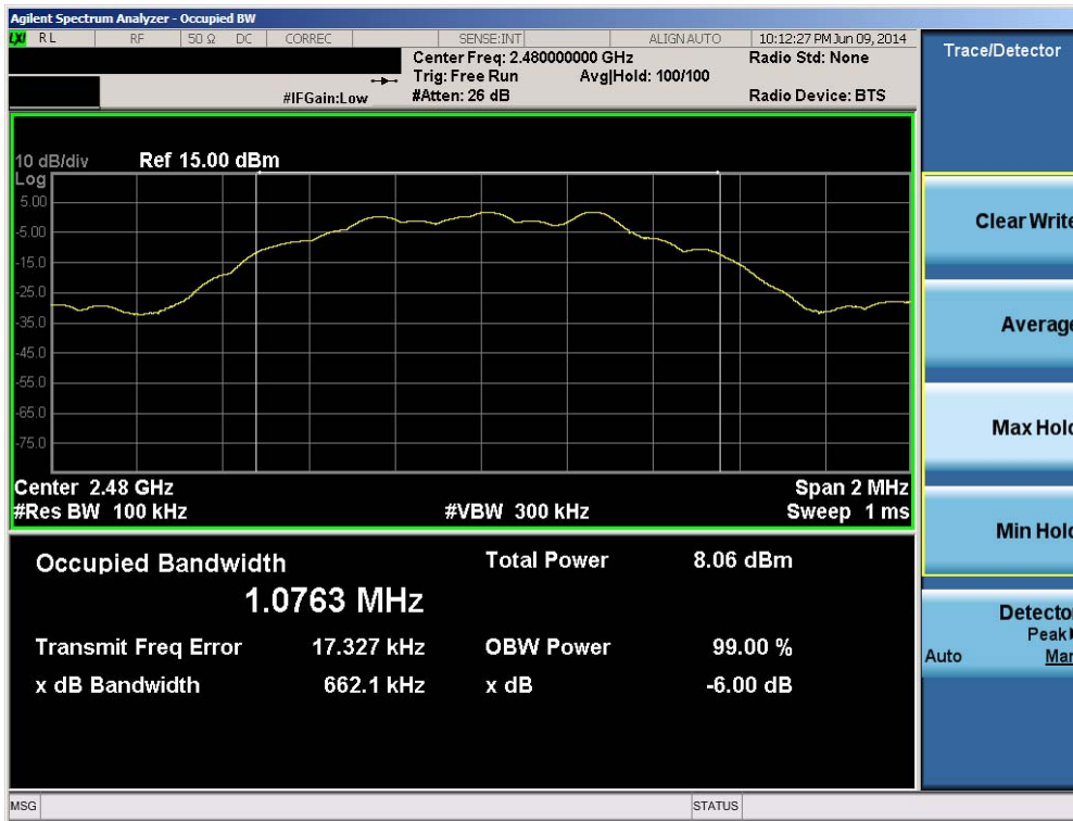
Plot 6-3. 6dB Bandwidth Plot (Bluetooth (LE) – Ch. 39)
