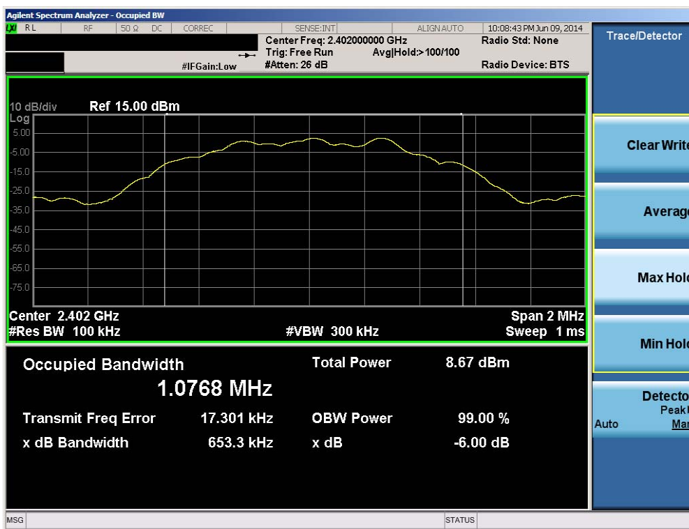
Plot 6-1. 6dB Bandwidth Plot (Bluetooth (LE) – Ch. 0)
