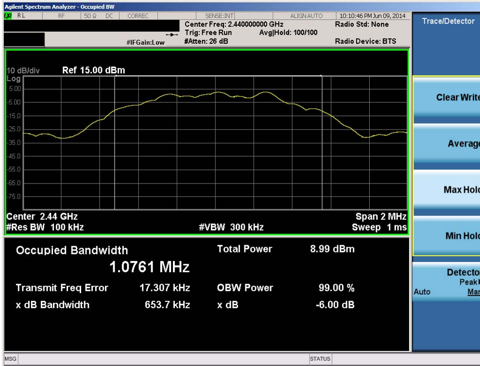
Plot 6-2. 6dB Bandwidth Plot (Bluetooth (LE) – Ch. 19)
