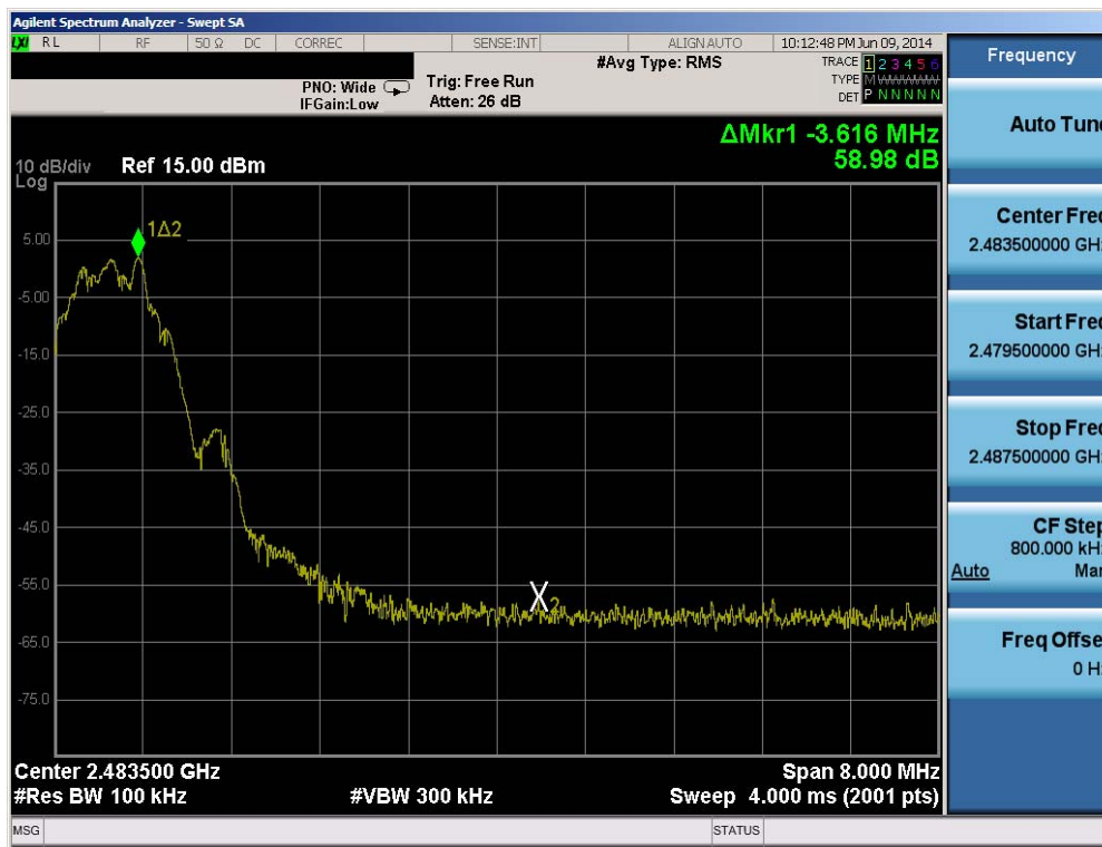
Plot 6-11. Band Edge Plot (Bluetooth (LE) – Ch. 39)
