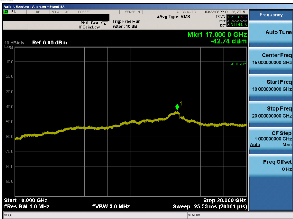
Plot 7-13. Conducted Spurious Plot (Band 4 – 15.0MHz QPSK – RB Size 1, RB Offset 0 – High Channel)
