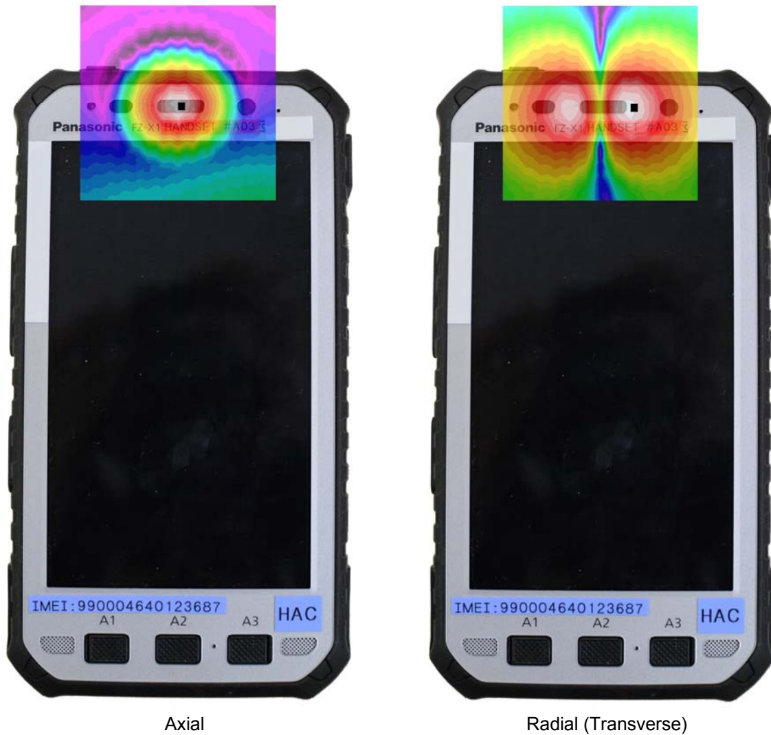
Figure 12-3 T-Coil Scan Overlay Magnetic Field Distributions
