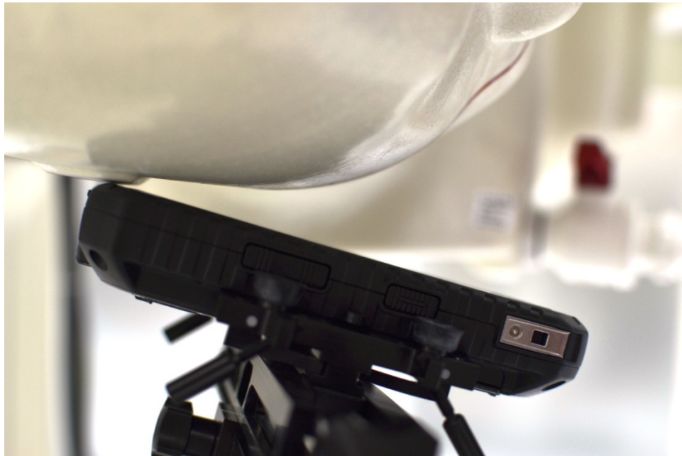
SAR Test Setup Photo 2: Right Tilt
