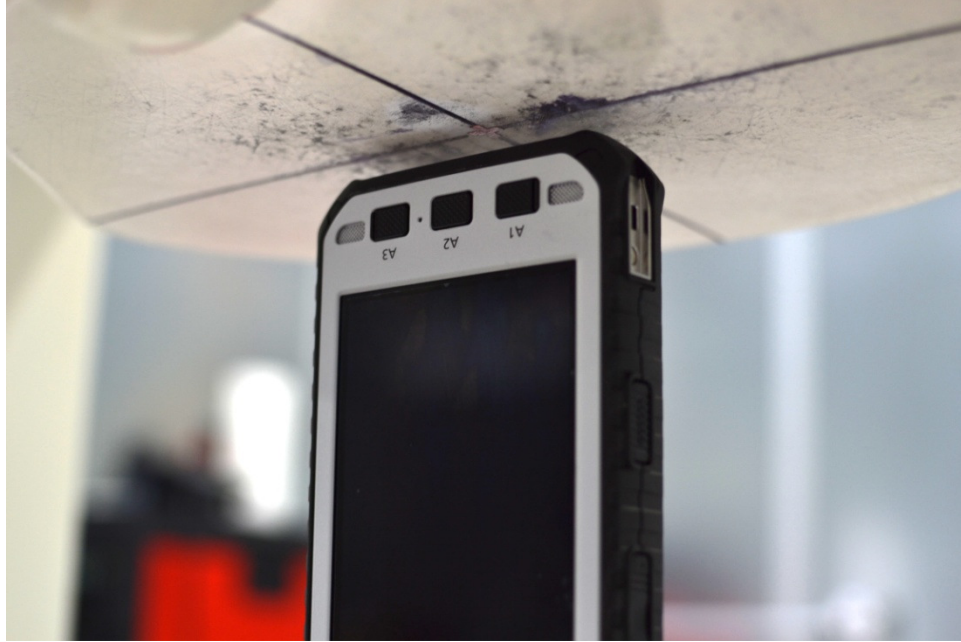
SAR Test Setup Photo 13: Bottom Edge at 1.0 cm
