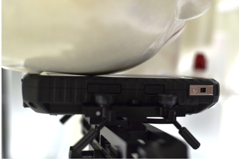
SAR Test Setup Photo 1: Right Cheek
