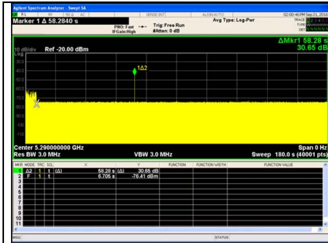
Radar at end of CAC – VHT80 – 5290MHz
