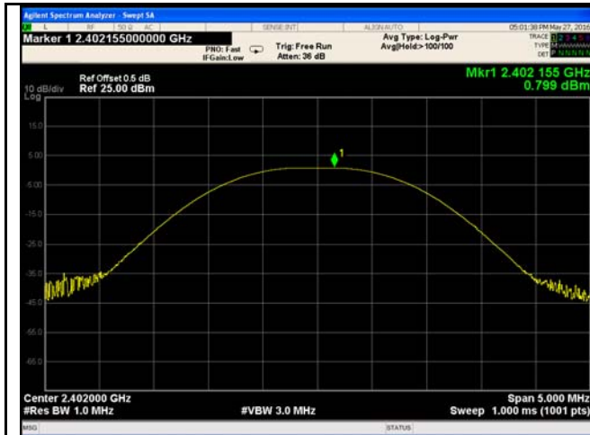
GFSK Output power - Low CH 2402
