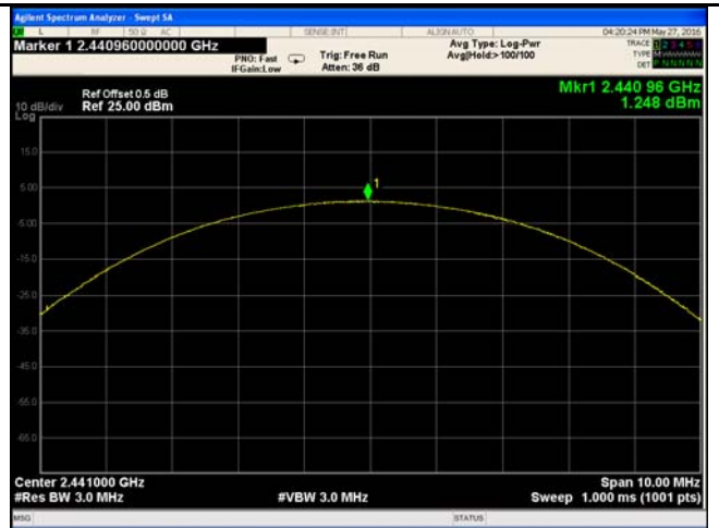
8DPSK Output power - Mid CH 2441
