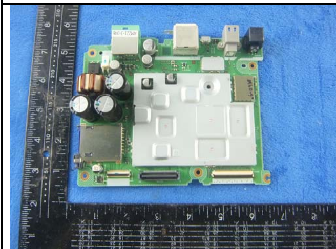
AM221-3-046 board with Shielding - Front View
