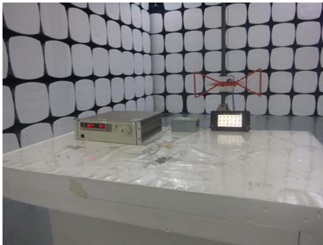
Radiated Spurious Emissions Test Setup Below 1GHz
