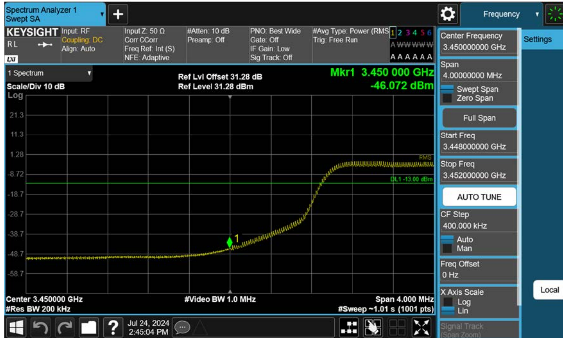
LTE B42_20 M_Band Edge_Low_QPSK_Full RB (1)
