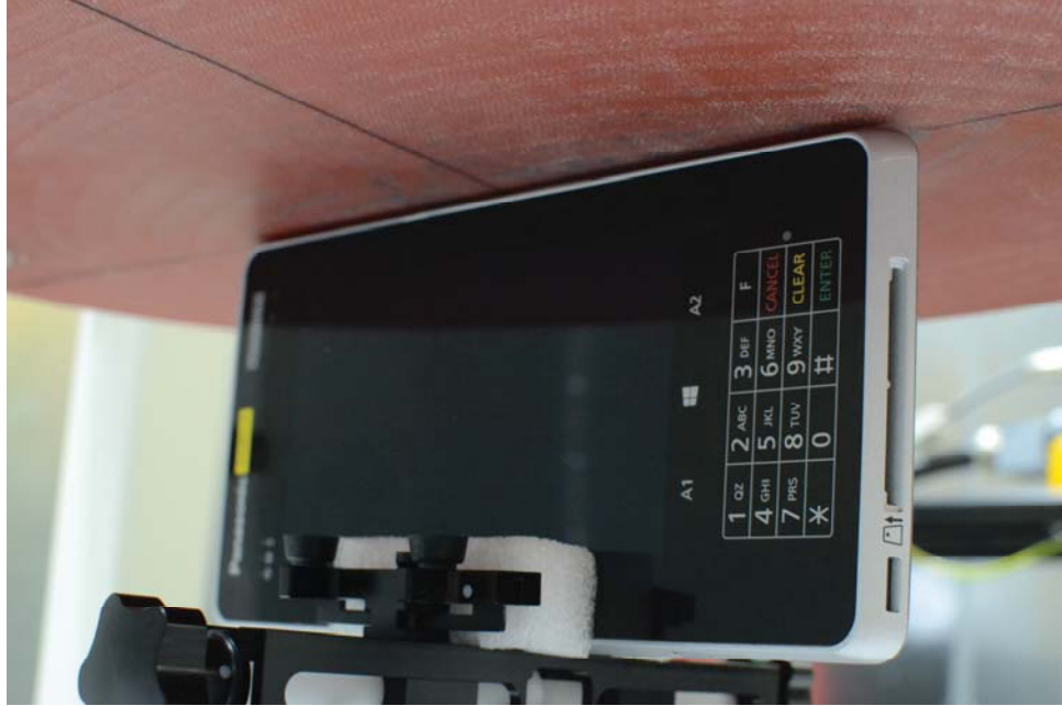
SAR Test Setup Photo 7: Right Edge (Perpendicular) at 0.0 cm
