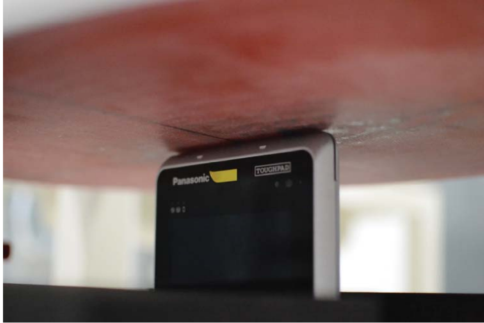
SAR Test Setup Photo 3: Top Edge (Perpendicular) at 0.0 cm
