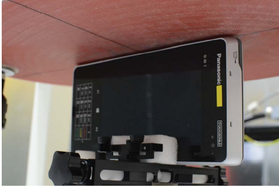
SAR Test Setup Photo 11: Left Edge (Perpendicular) at 0.0 cm
