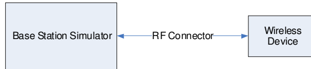
Figure 8-1 Power Measurement Setup
