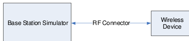
Figure 8-2 Power Measurement Setup
