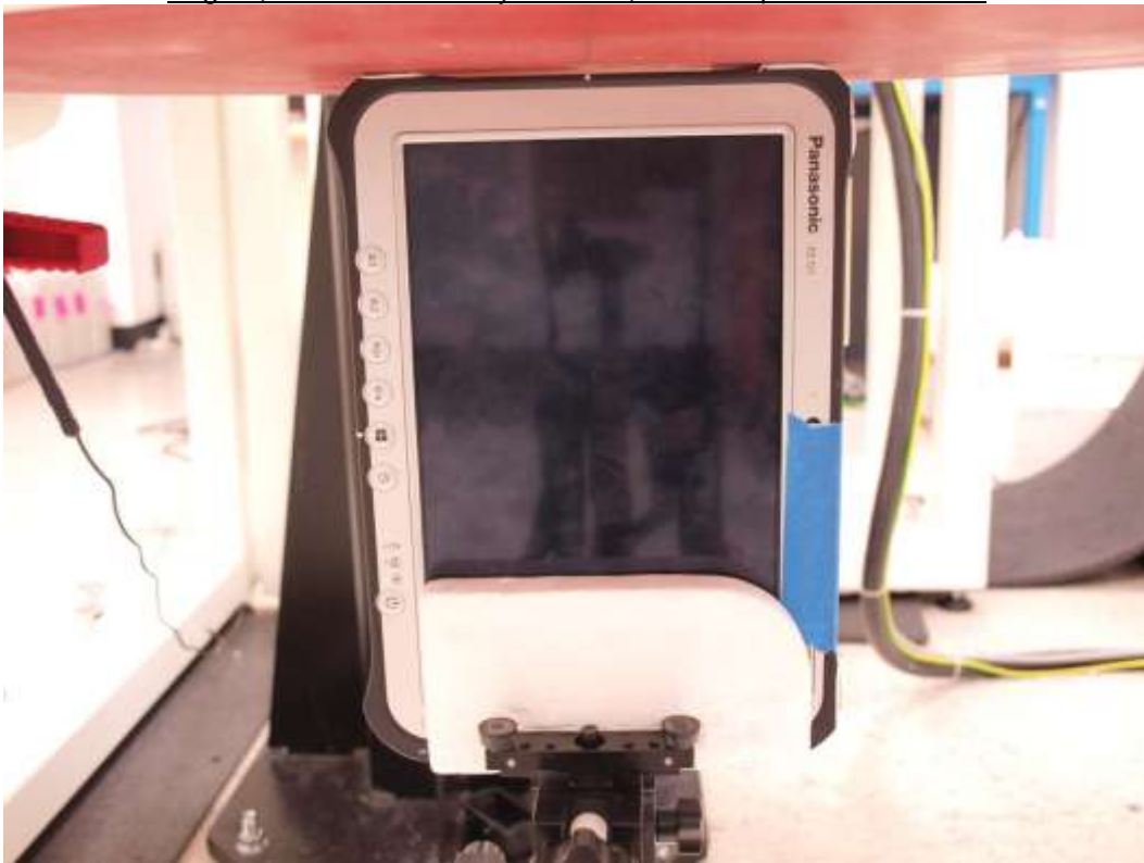
Edge 4, Main and Auxiliary Antenna, 0 mm Separation Distance
