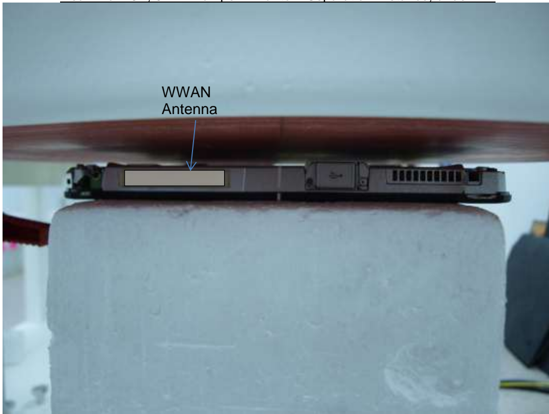
Edge 1 Prox. Off, 20 mm Separation Distance
