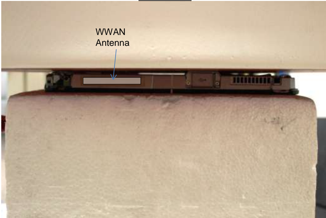
Edge 1 Prox. On, 0 mm Separation Distance
